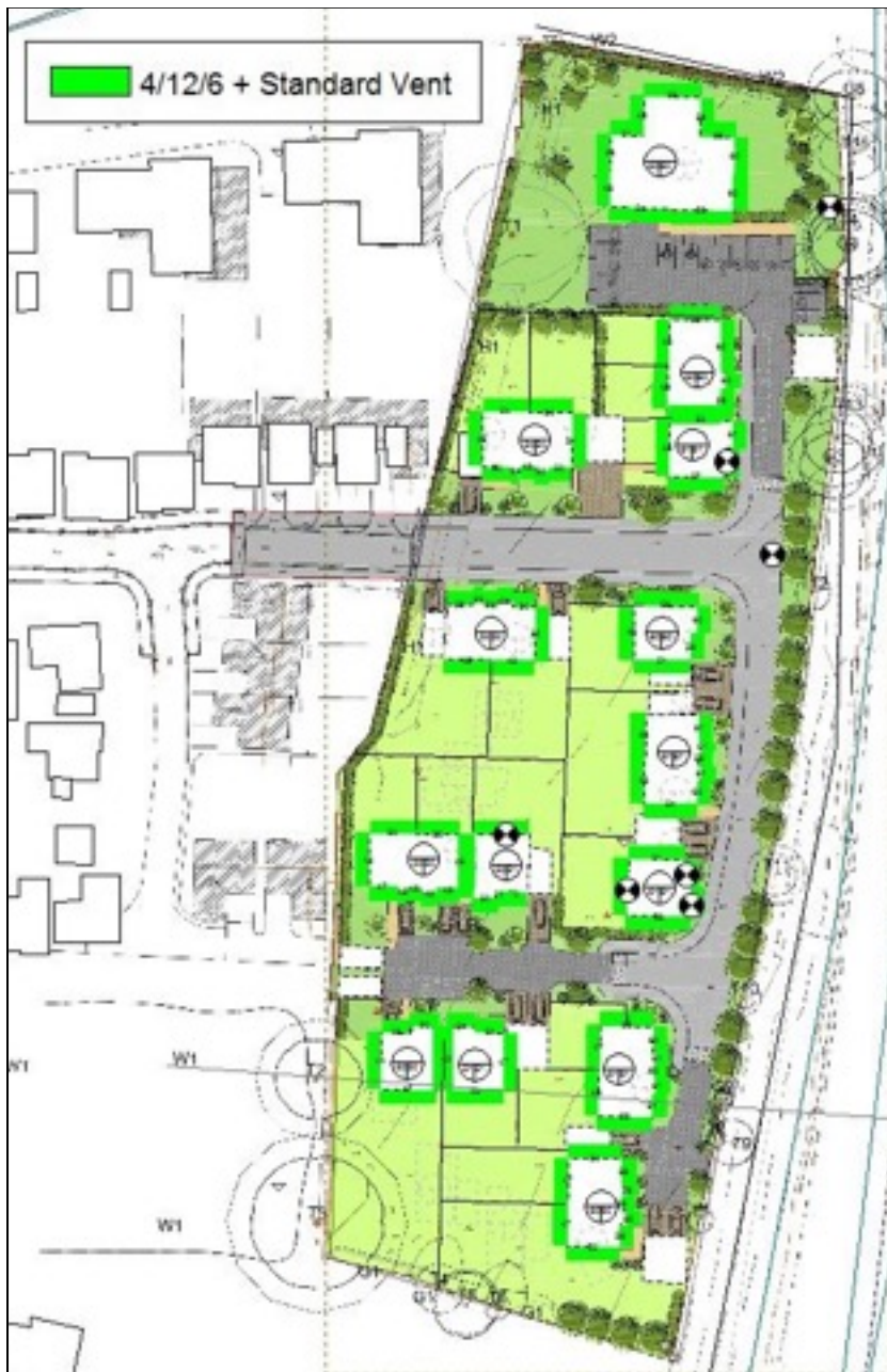
Figure B1: Proposed Glazing And Ventilation Strategy with 3m Barrier
