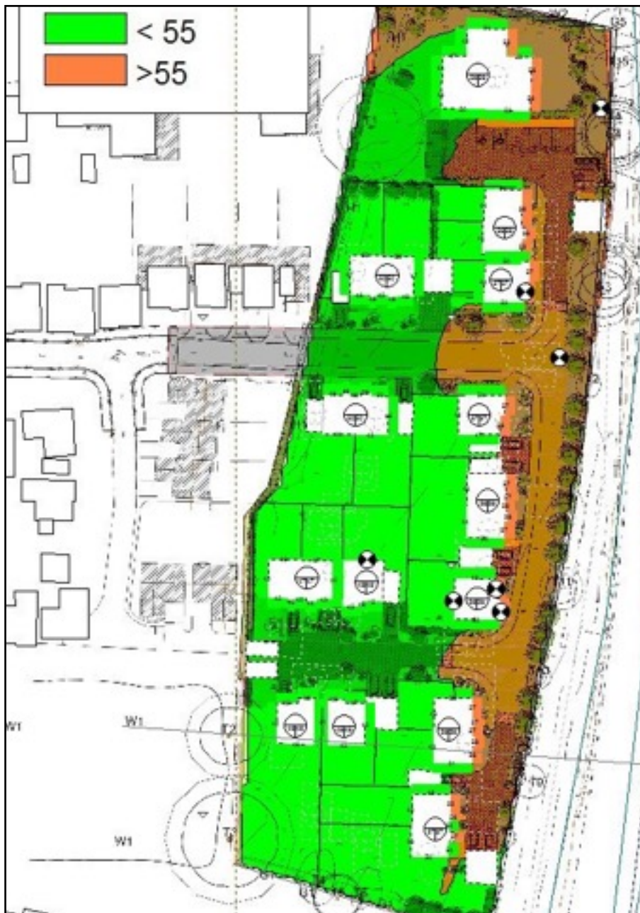
Figure B2: Predicted Garden Noise Level with 3m Barrier
