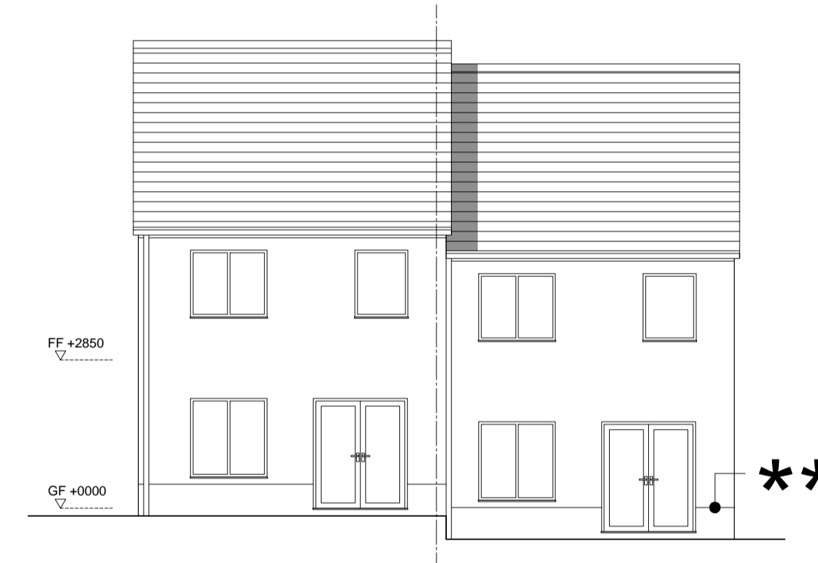
REAR ELEVATION Note: Step between dwellings vary
