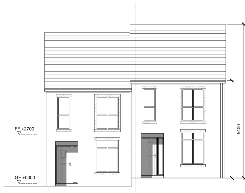
FRONT ELEVATION - PLOT NO. 10, 11, 12, 13, 14, 17, 18, 19, 20, 116, 117, 135, 136, 163, 164, 171, 172, 175, 176, 179, 180, 185, 186 (LIGHT BRICK)
