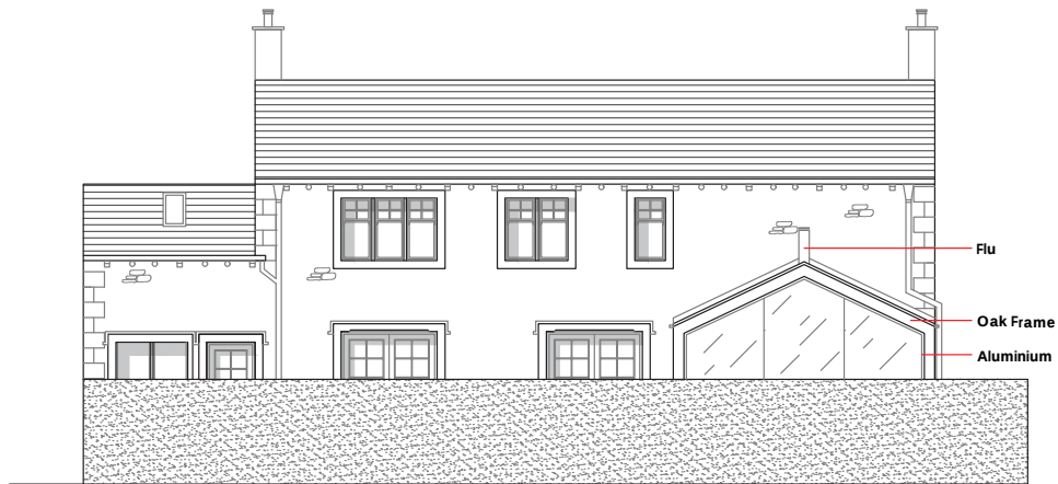
NORTH WEST ELEVATION
