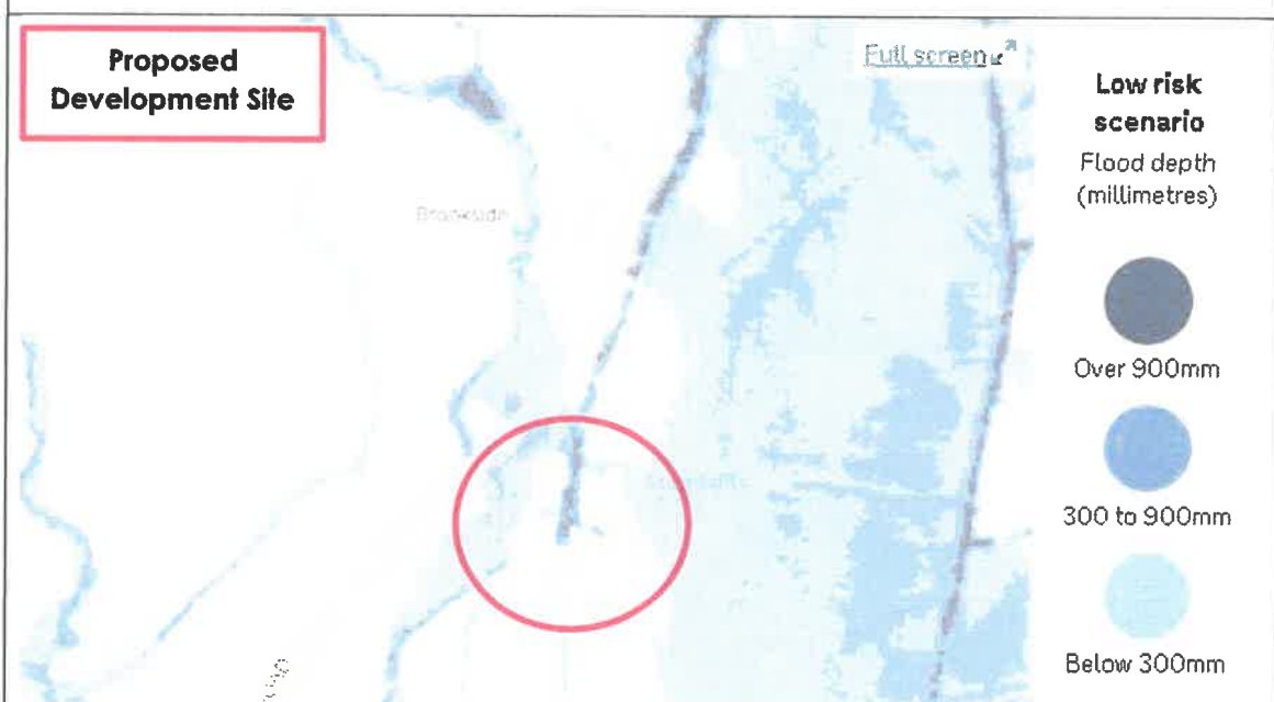
Figure 6.5: Surface Water Depth – Low Probability Event Depth
