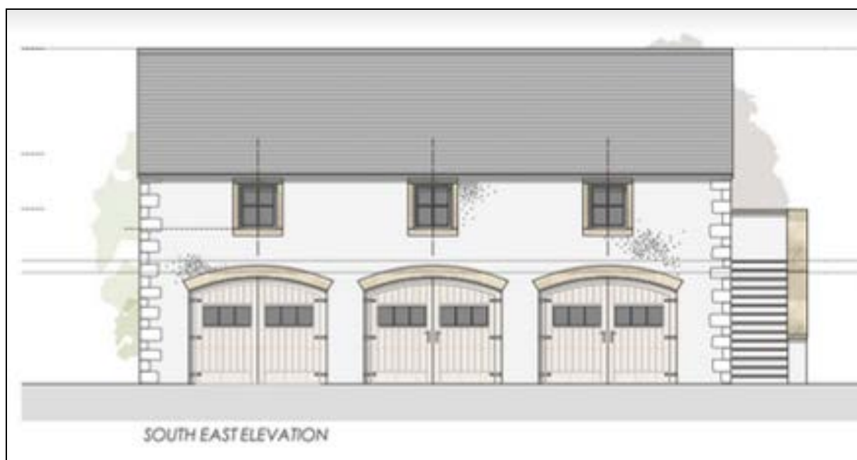
Figure 3. Proposed front elevation of the garage
