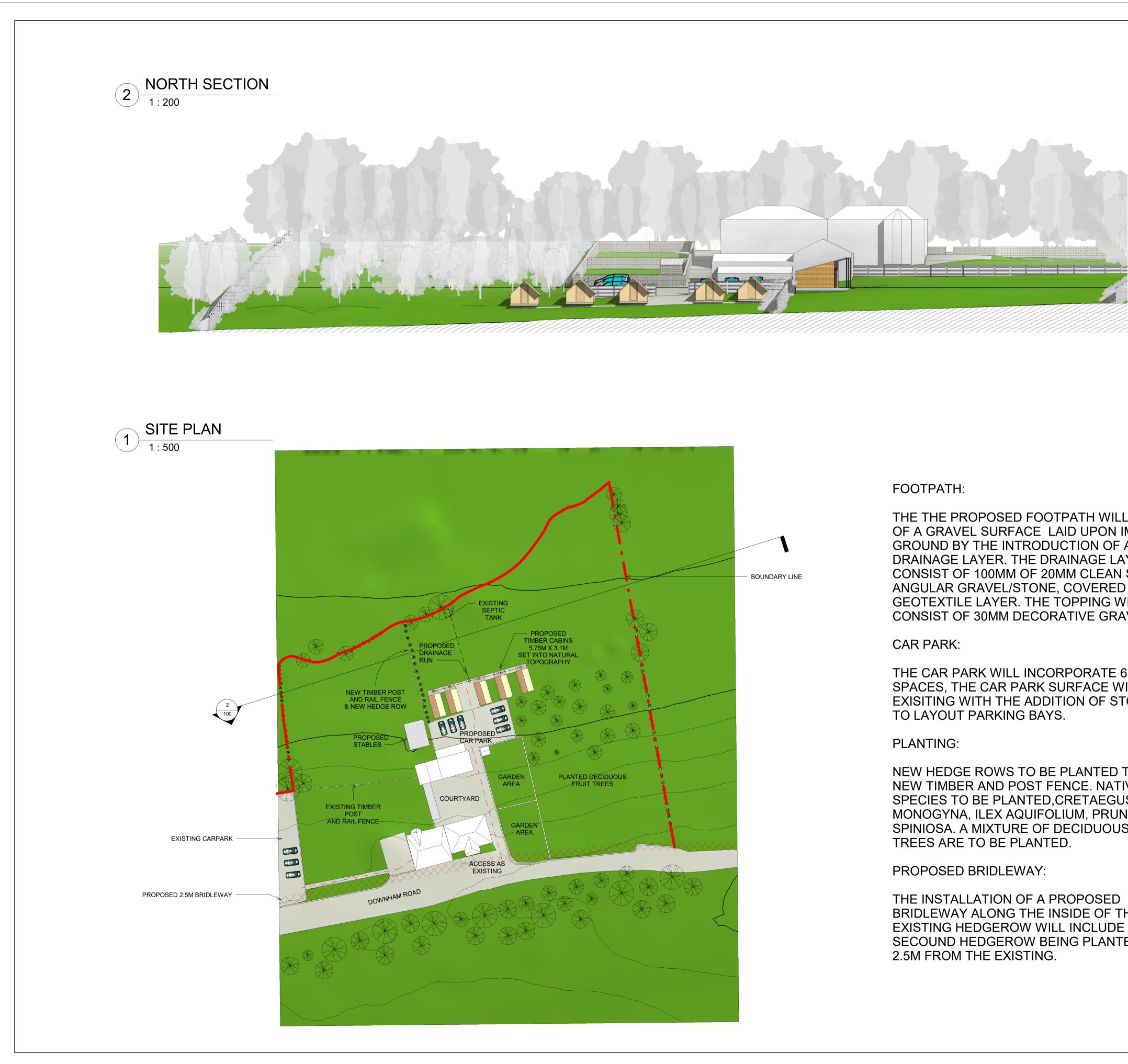
THE THE PROPOSED FOOTPATH WILL CONSIST OF A GRAVEL SURFACE LAID UPON IMPROVED GROUND BY THE INTRODUCTION OF A DRAINAGE LAYER. THE DRAINAGE LAYER WILL CONSIST OF 100MM OF 20MM CLEAN SHARP ANGULAR GRAVEL/STONE, COVERED WITH A GEOTEXTILE LAYER. THE TOPPING WILL CONSIST OF 30MM DECORATIVE GRAVEL.
