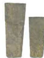
Swept valley slip slates
