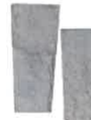
Swept valley slip slates
