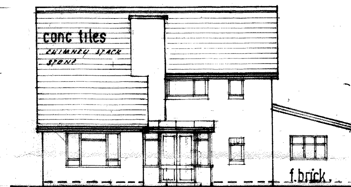
existing front elevation
