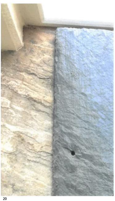
Image above shows proposed new roof grey slate tile
