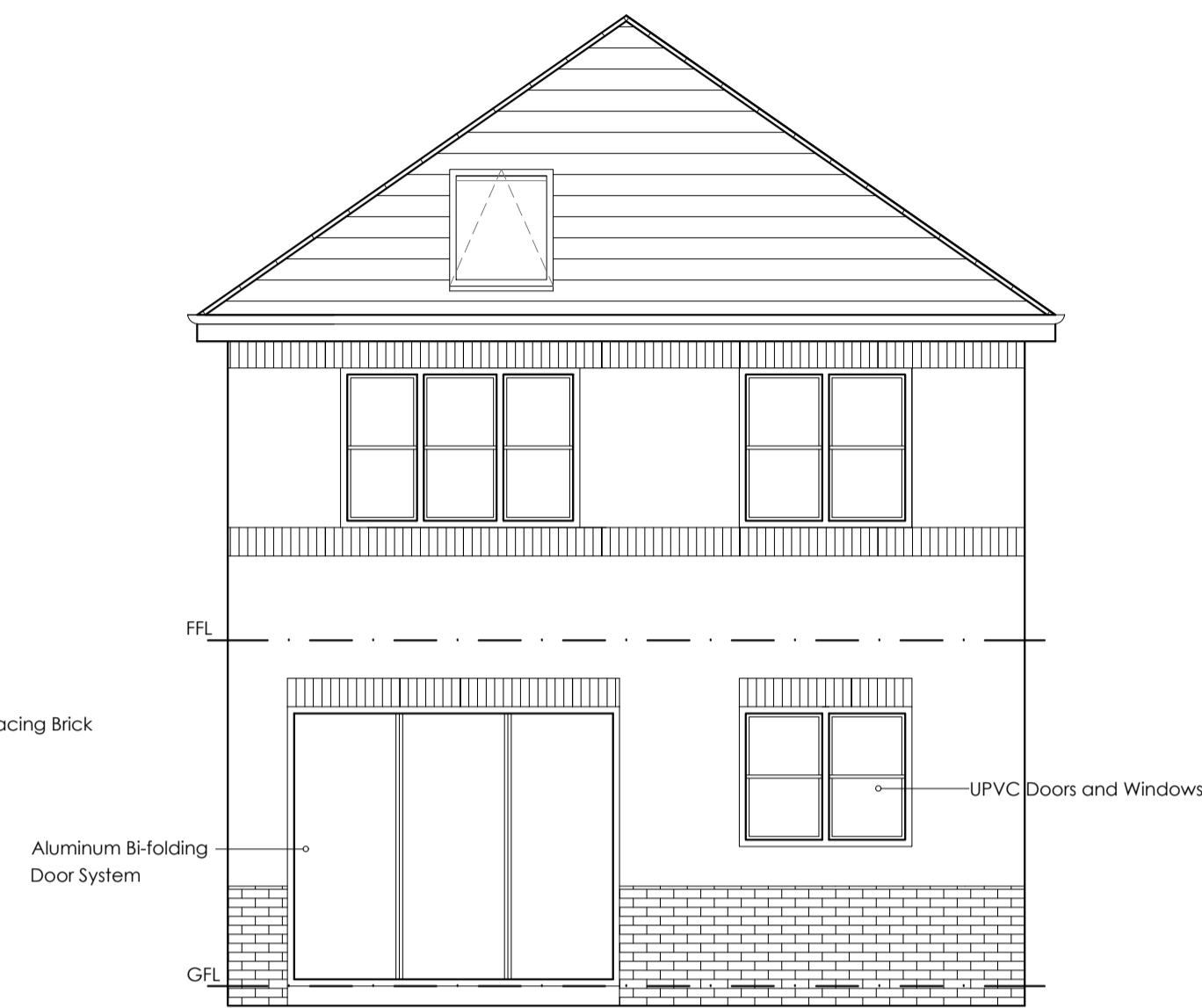
Proposed South West Elevation Scale 1:50
