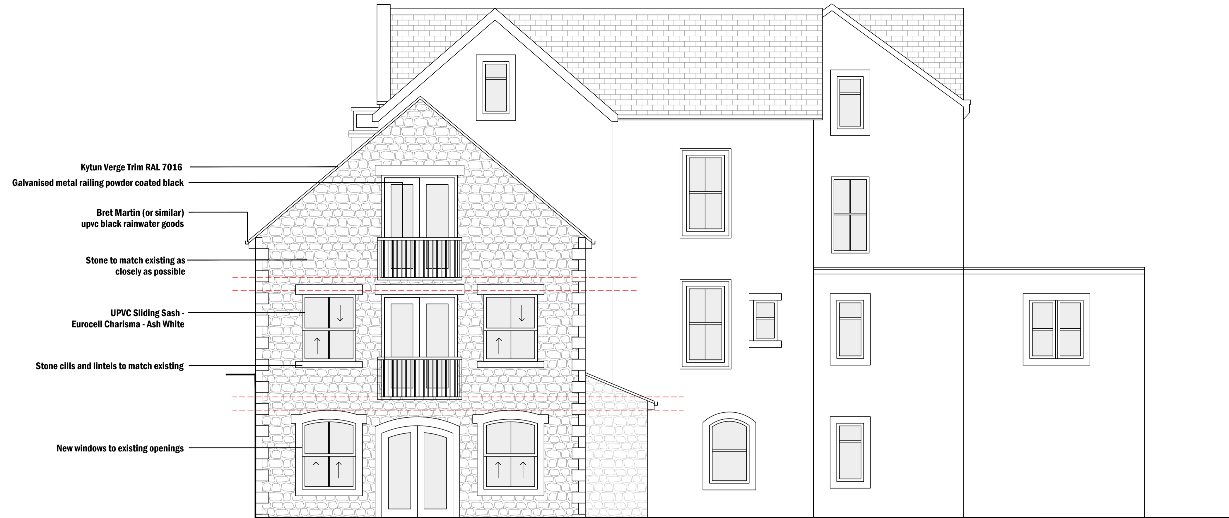
PROPOSED END ELEVATION 1:50
