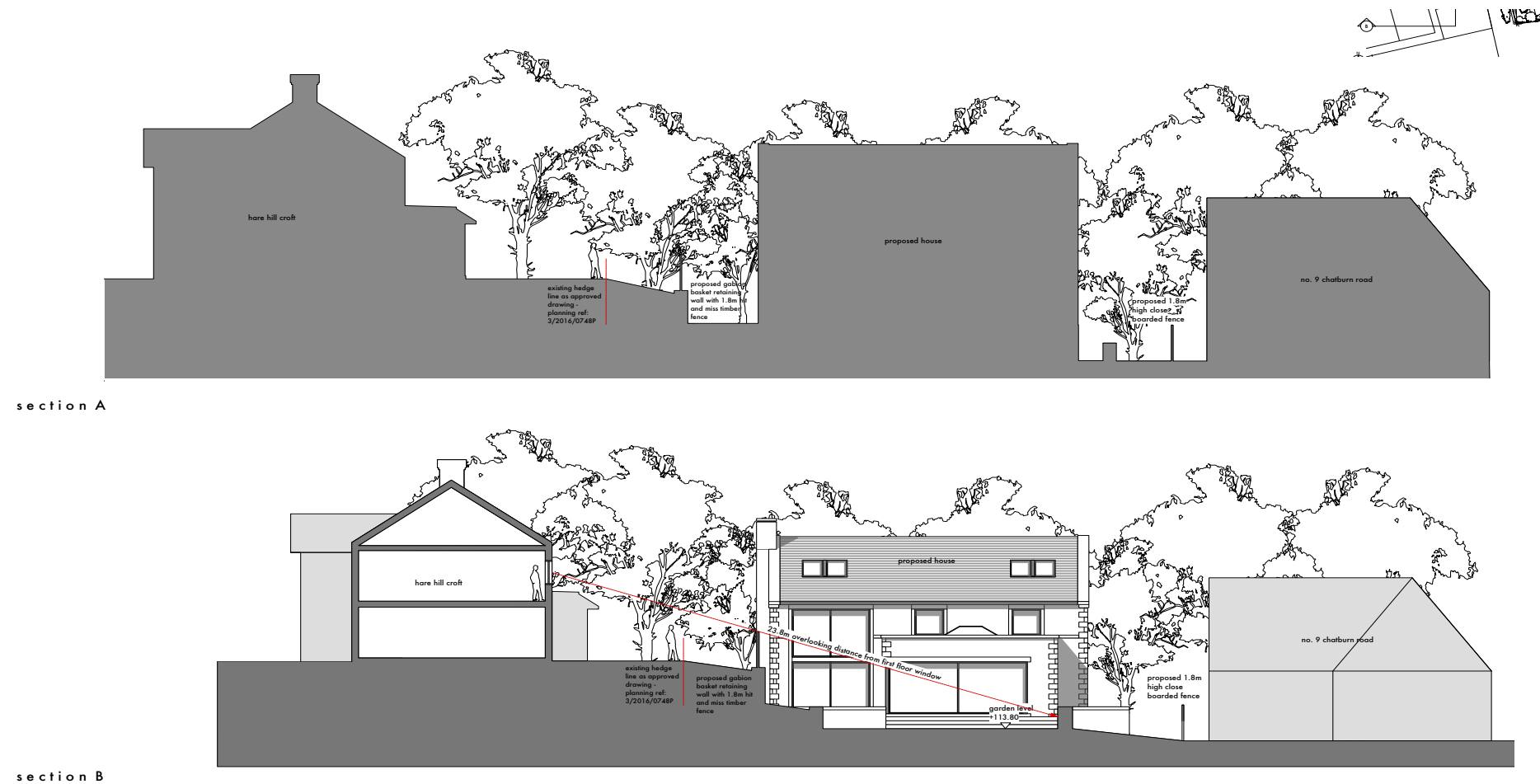
sections to show overlooking distance
