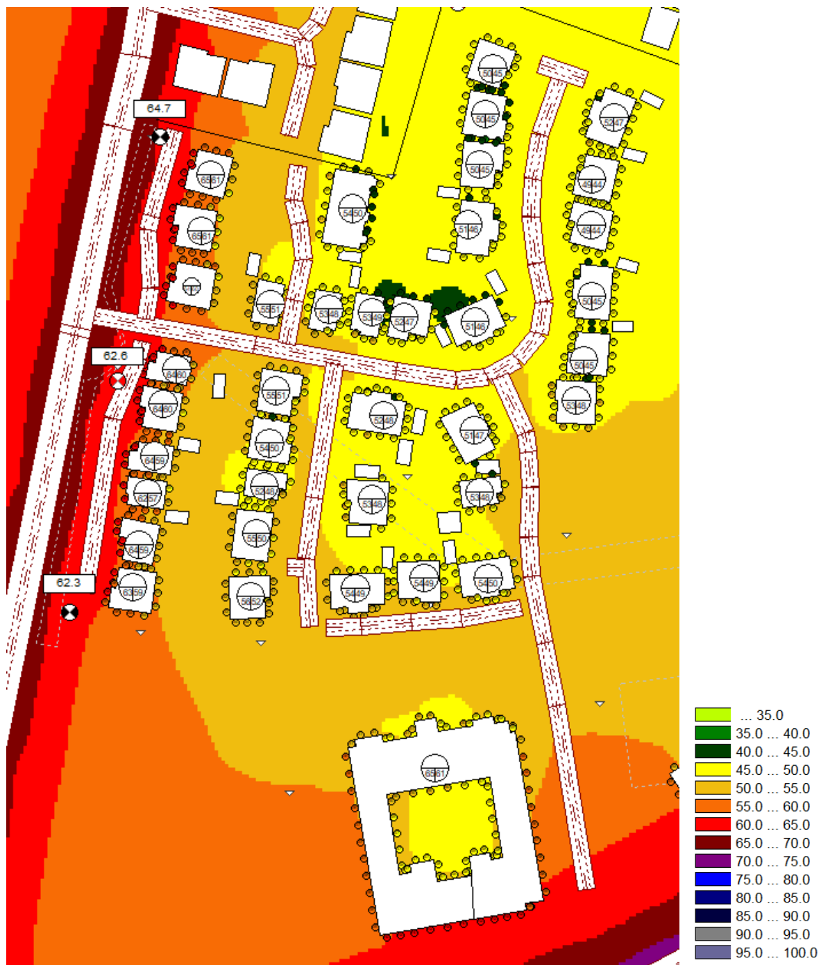
Figure 6 Daytime noise levels across proposed site (.5m above the ground) - dB L_{Aeq,16h}
