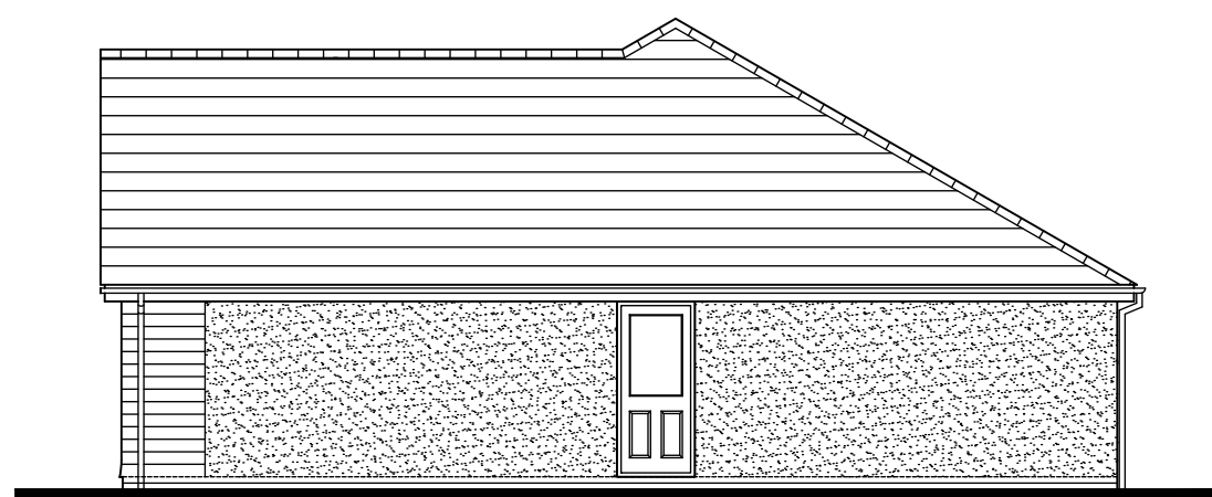
SIDE ELEVATION - TUDOR BOARDED 1:100
