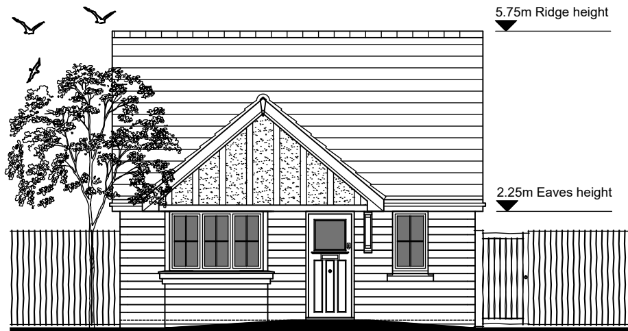
FRONT ELEVATION - TUDOR BOARDED 1:100
