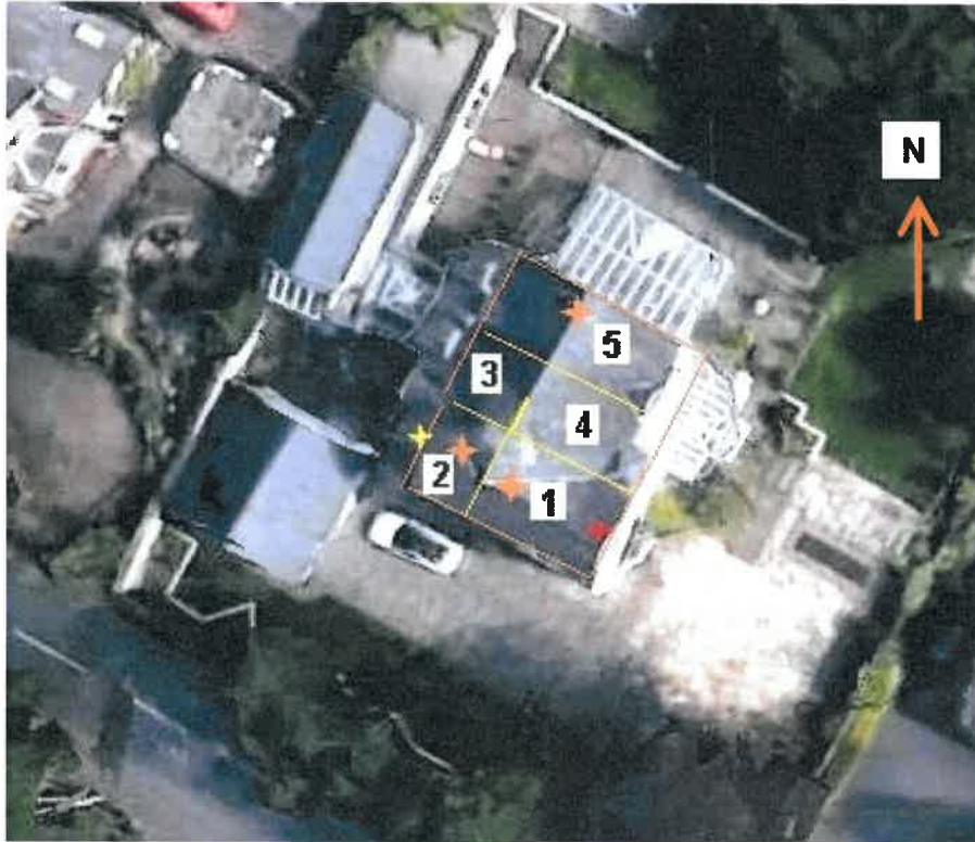
Fig. 2. Main roof outlined in orange, with subdivisions roughly illustrated in yellow. There are crawl-openings between zones 1 and 4, 1 and 2 and 3/4 and 5. Largest collection of droppings illustrated by red cross. Smaller collections beneath defects in felt shown by orange crosses. The small-scale distribution of droppings is much wider however, especially under the ridge beam of 1. Zones 3 and 4 contain few droppings. Location of droppings on external gable wall illustrated by yellow cross. The proposed extension is at the north-east-facing gable (zone 5)
