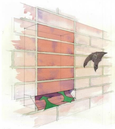
Insert 2: Example of an integral bat box. The outer leaf can be clad to match the stone elevations (available from http://www.habibat.co.uk )
