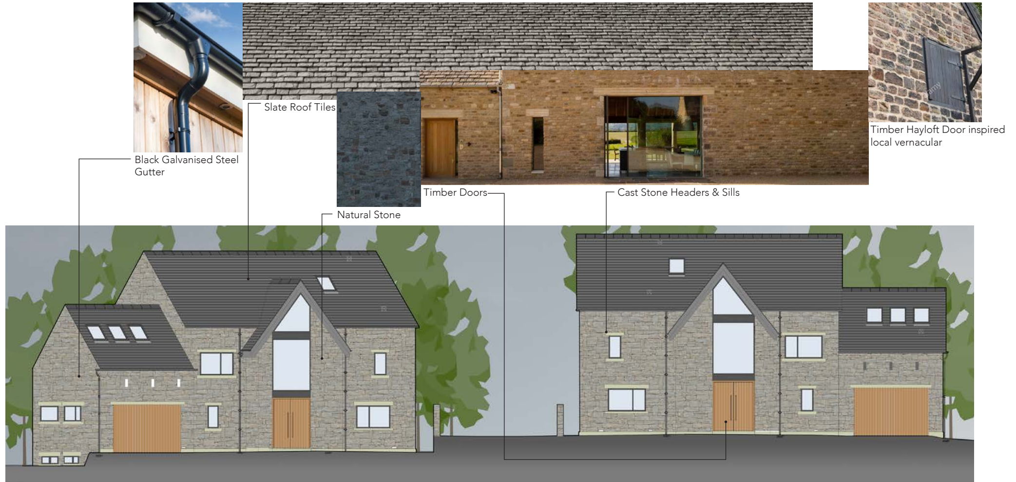
FIG 21 - Proposed Site Elevation
