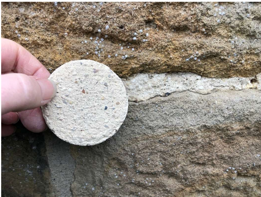
Photo 5 - Proposed "Pale Yellow" lime mortar from Mike Wye Ltd to match existing
