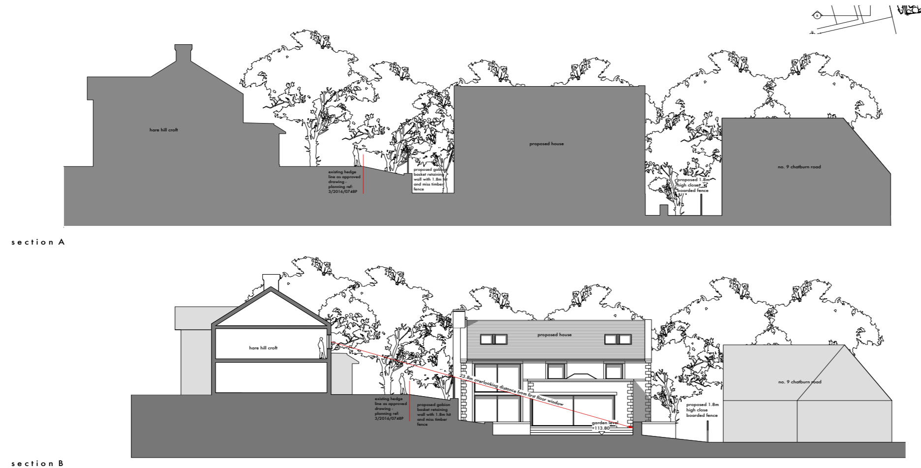
sections to show overlooking distance
