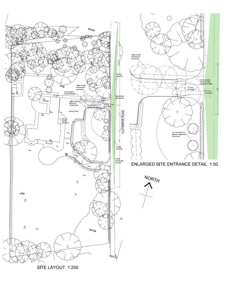
Rev A: Trees removed & 2No limes added, entrance moved southwards by 3.5m, visibility splay7 added
