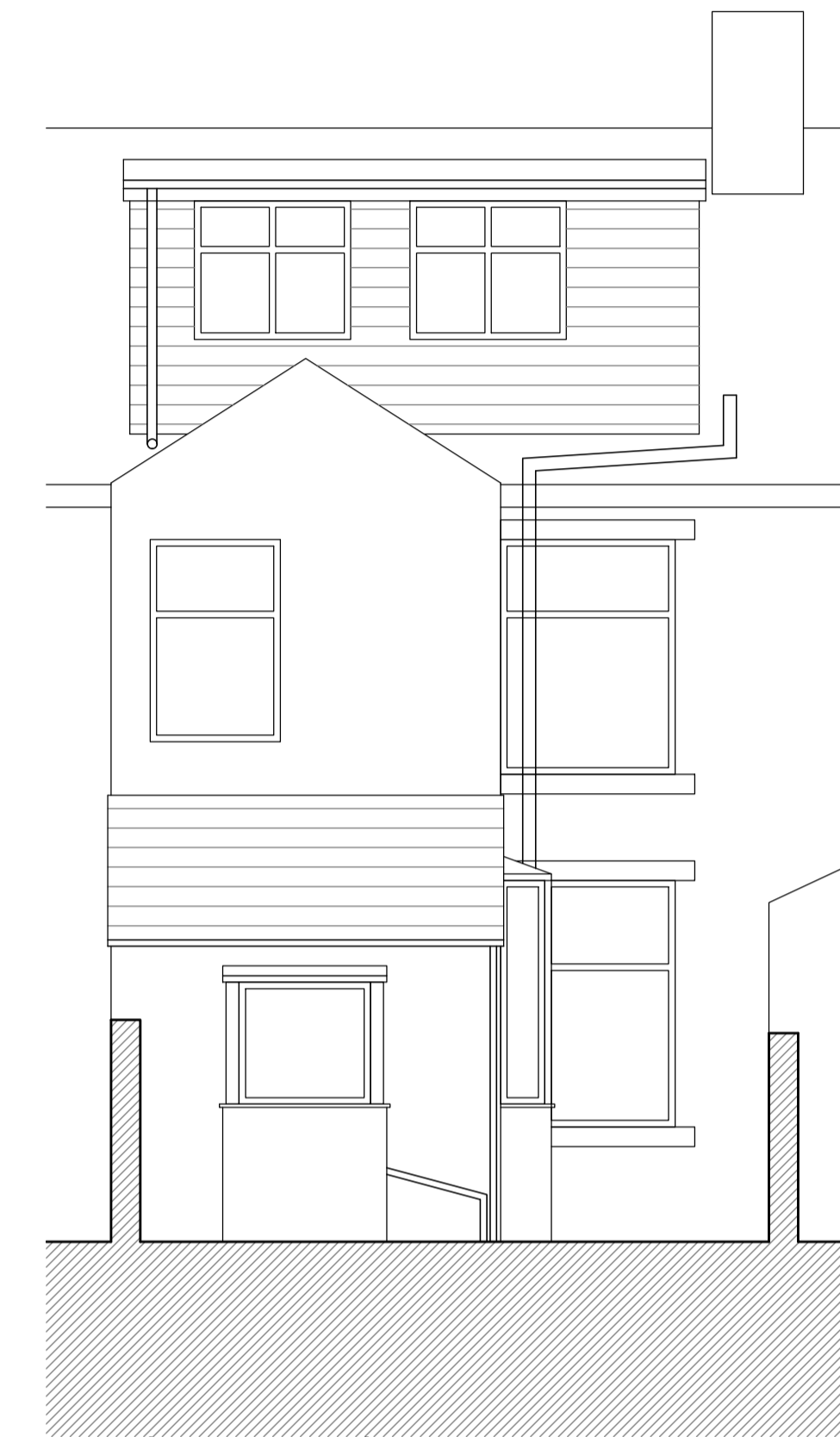
Rear Elevation (yard)
