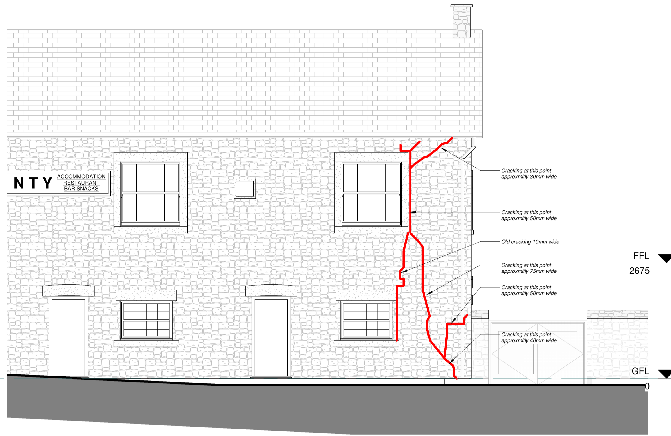
Existing Part Front Elevation Showing Damage 1 : 50
