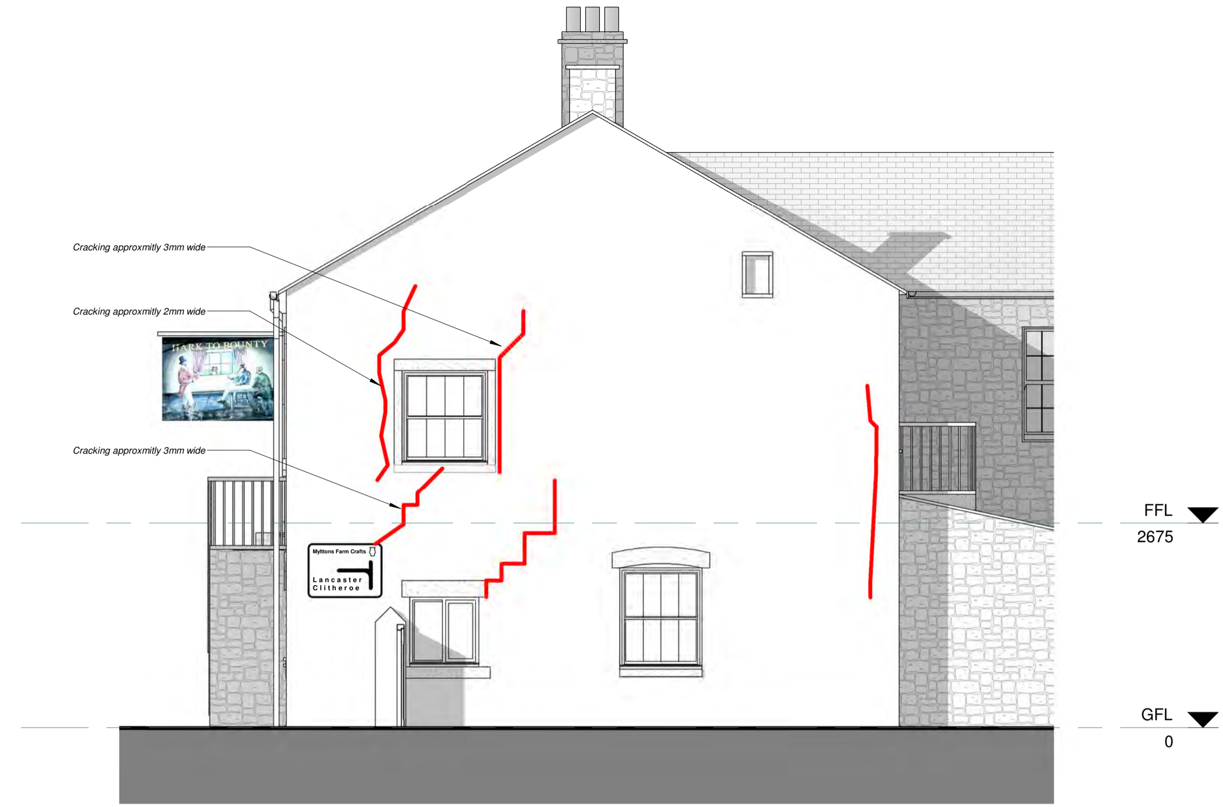
Existing Part Side 1 Elevation Showing Damage 1 : 50
