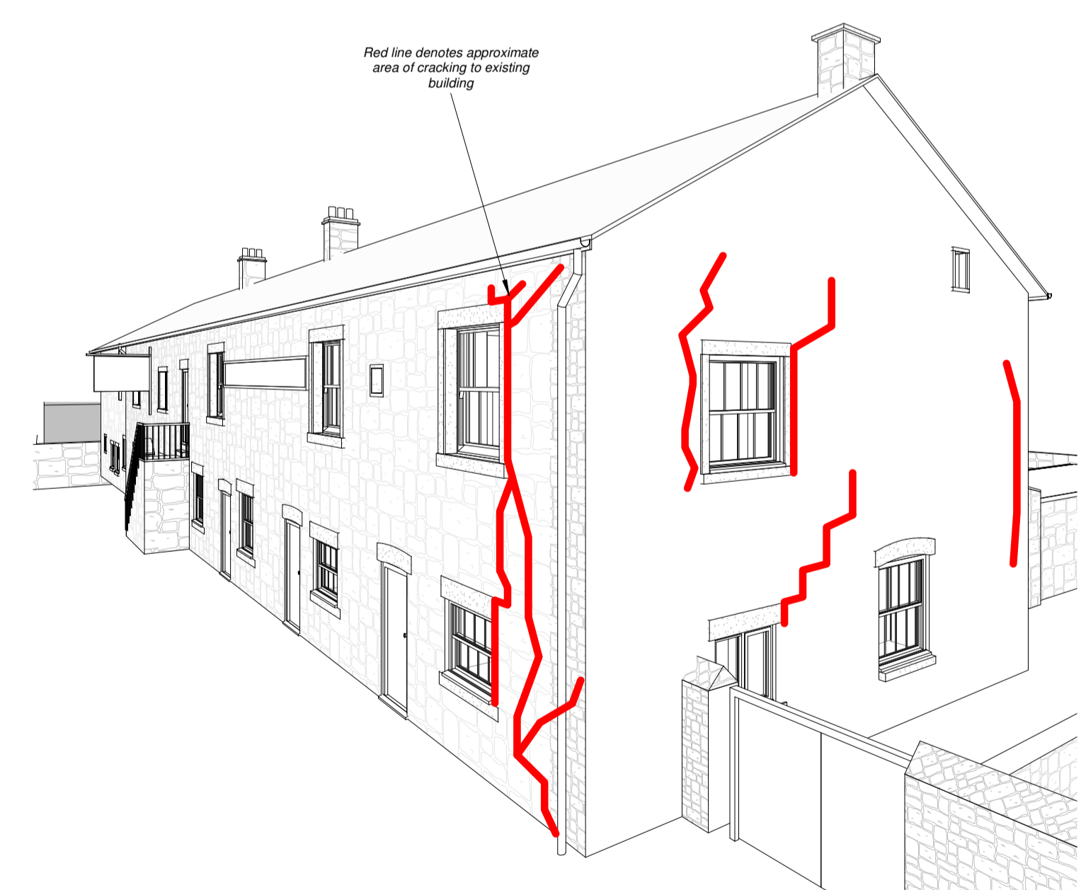
3D View Identifying Damage To Building
