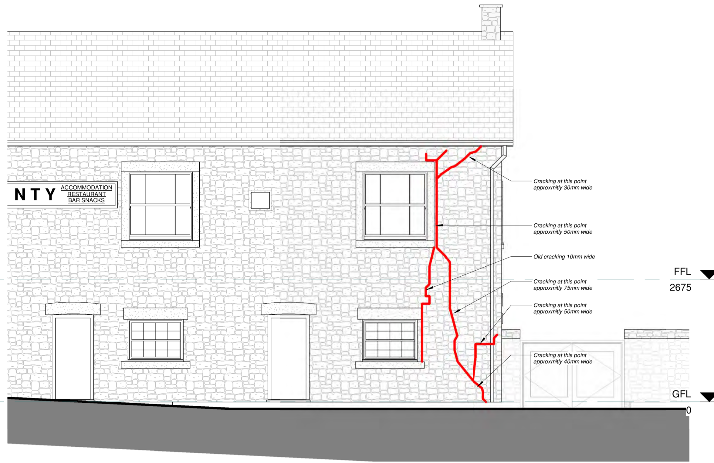
Existing Part Front Elevation Showing Damage 1 : 50
