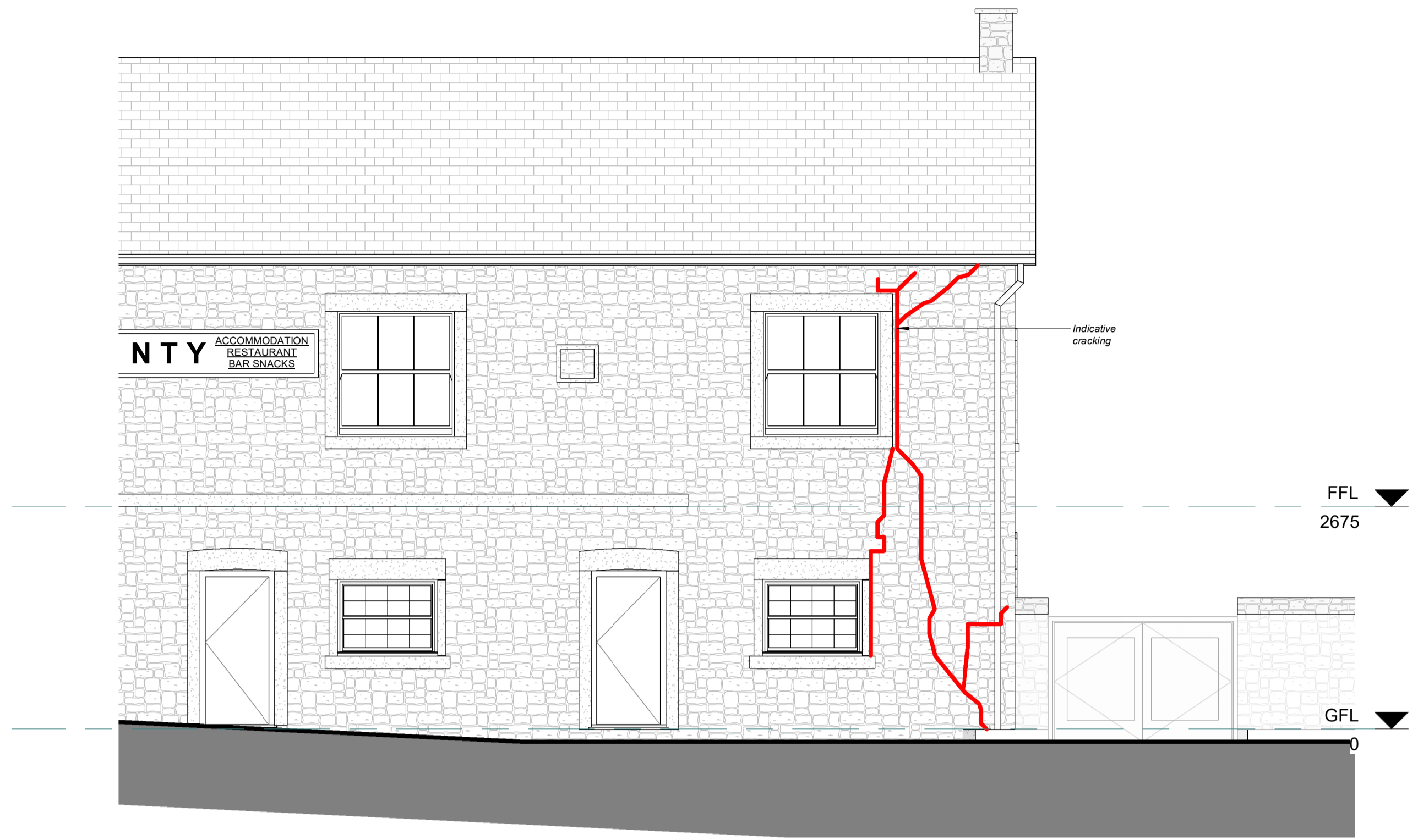
Existing Part Front Elevation Showing Damage 1 : 50
