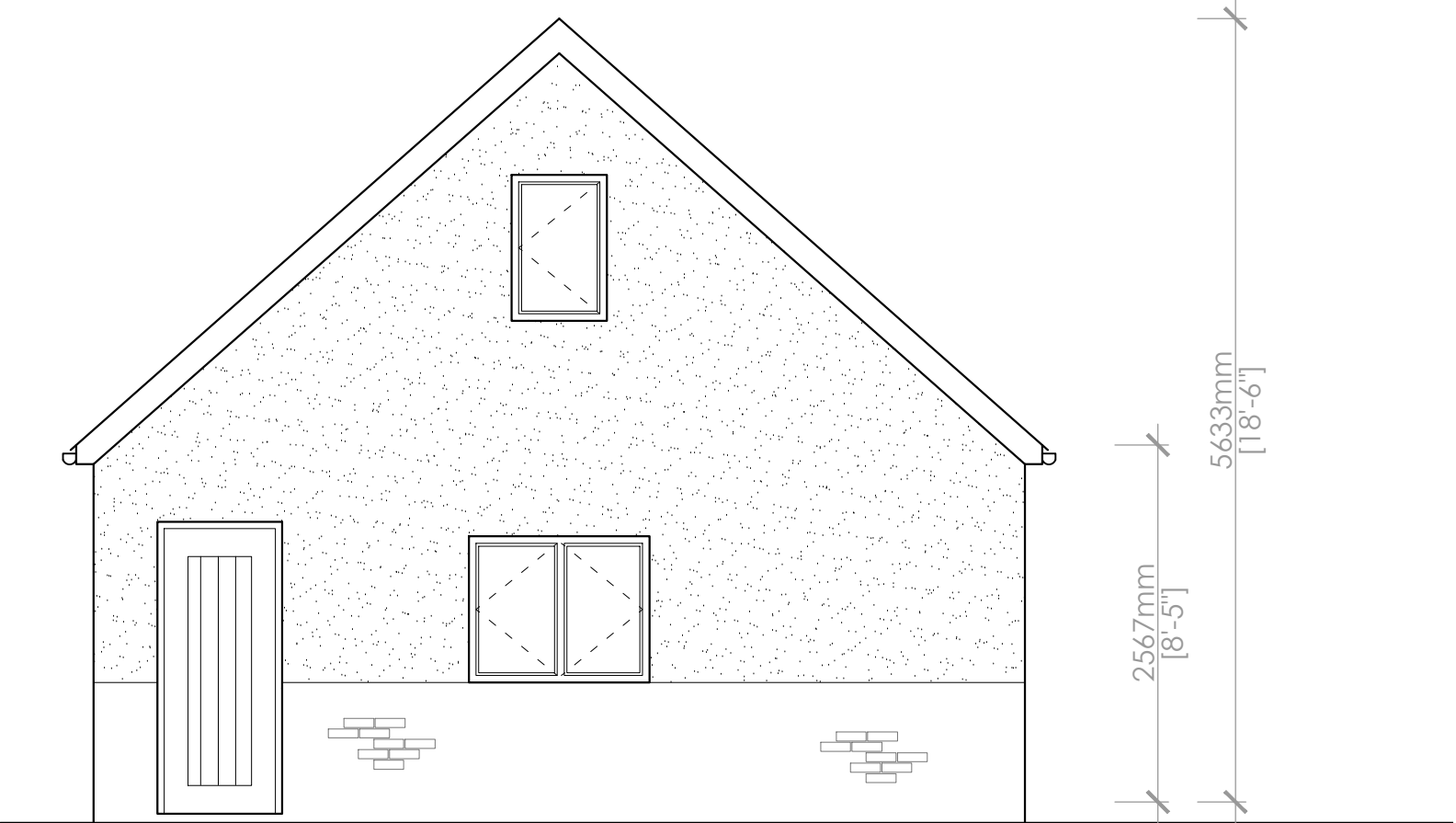
PROPOSED GARAGE SIDE / SECTION ELEVATION SCALE 1:50
