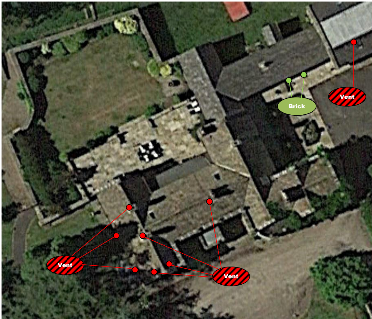
Figure 10 - Shows the location on the site layout of the proposed access vents (red and black) and bat brick (green) access mitigation
