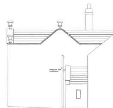
Proposed North Elevation inside the courtyard showing one new s&vp connection
