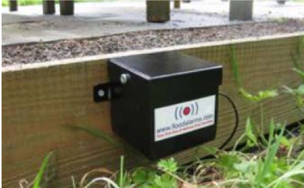
Figure 7.3: Stand Alone Flood Alarm Example
