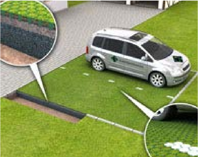
Spa car park - 49 spaces Reinforced grass system - Geosynthetic Golpla or similar. Perimeter screening to be indigenous woodland species including new length of hedgerow in keeping with local field pattern and size.
