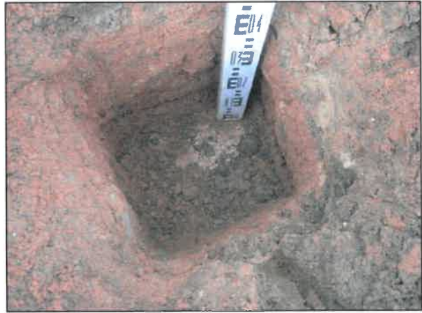
Photographs 13 & 14: Examples of validation photographs demonstrating inert cover depth and geotextile
