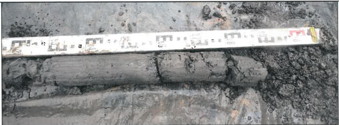
Photograph 10: Showing nature of pond infill materials within borehole WS04.
