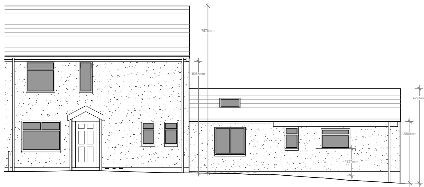
Front East Elevation 1:100
