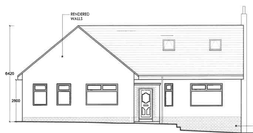
PROPOSED NORTH EAST FACING ELEVATION SCALE 1:100
