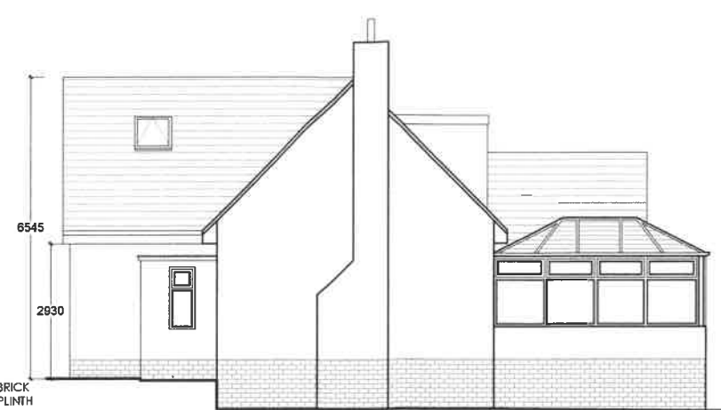
PROPOSED NORTH WEST FACING ELEVATION SCALE 1:100
