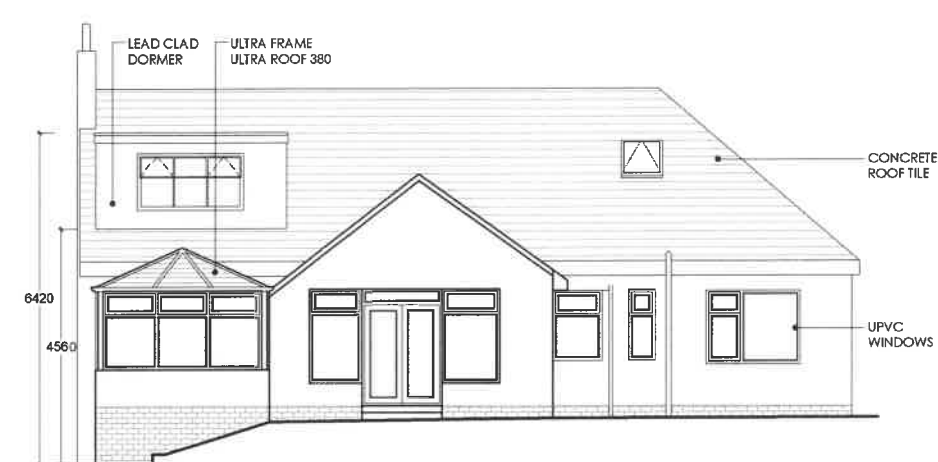
PROPOSED SOUTH WEST FACING ELEVATION SCALE 1:100
