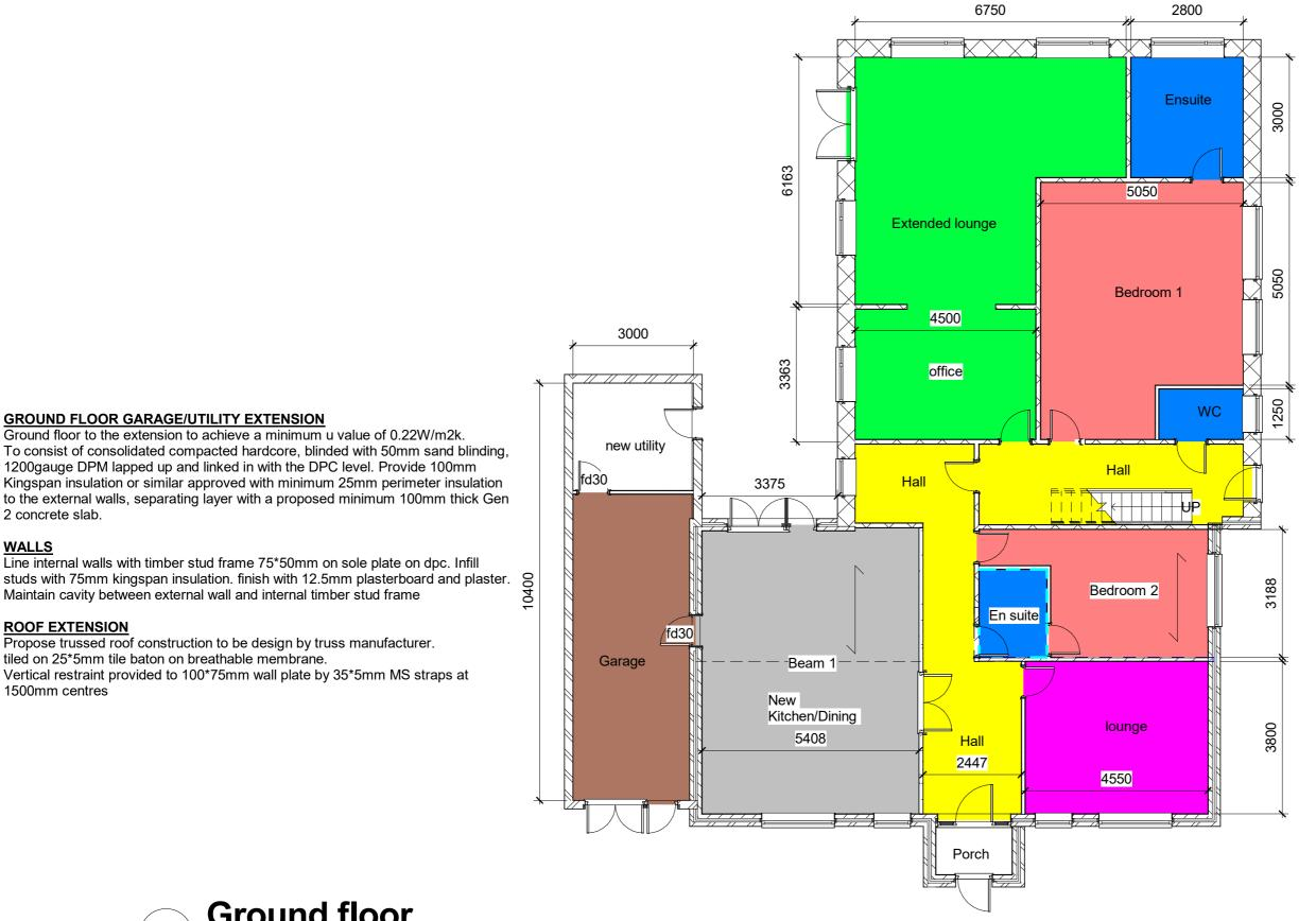
Line internal walls with timber stud frame 75\*50mm on sole plate on dpc. Infill Line internal walls with timber stud frame / 5 5011111 on sole plate on apo. .......
