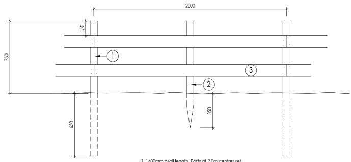
1. 1400mm o/all length. Posts at 2.0m centres set in augered hole and back filled with well rammed excavated material. Post to be 75x75mm treated larch rough sawn.
