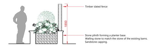
Cross section through boundary fence & planter Section AA 1/50scale
