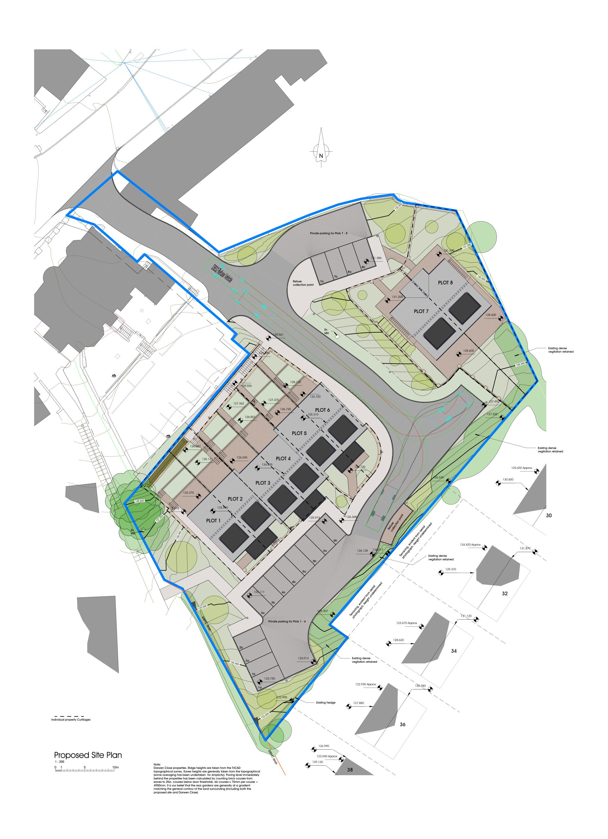
D 23-12-21 Approx. ground levels indicated to properties on Darwen Close. Terracing revised to plots 1 - 6. Plots 7 - 9 reduced by 1 unit C 30-09-21 Plots 1 & 2 patios/lawns revised. All drainage references removed
