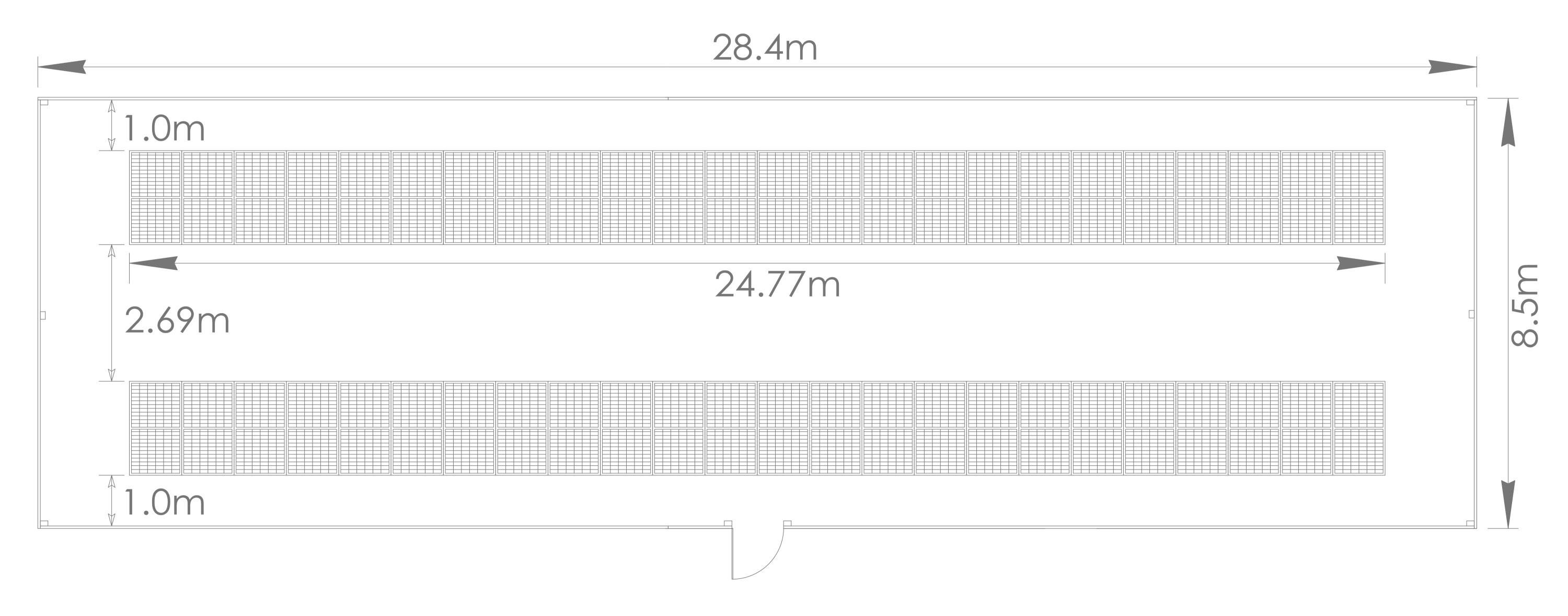
28.4 metre x 8.5 metre fenced area with gate 48 x Jinco solar panels in two rows of 24
