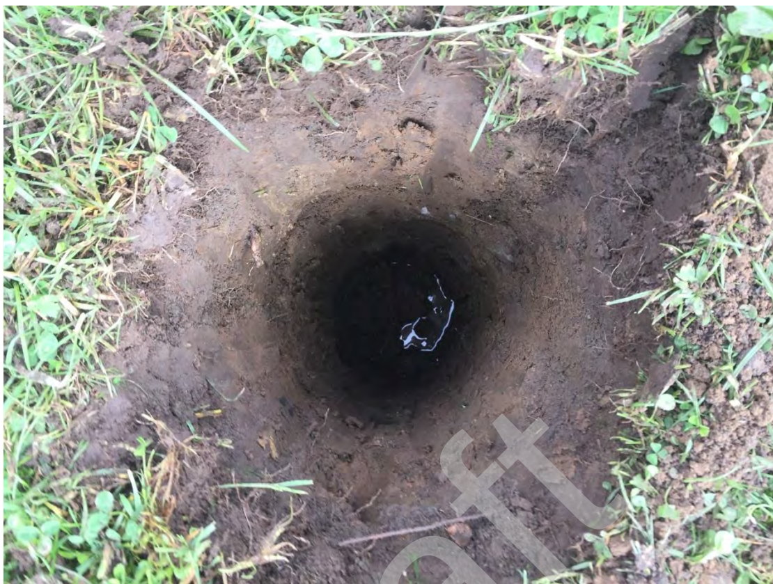
Figure 4. Borehole 1 (BH1). Ground water visible within the clay substrate at the base of the hand-dug portion of the hole.
