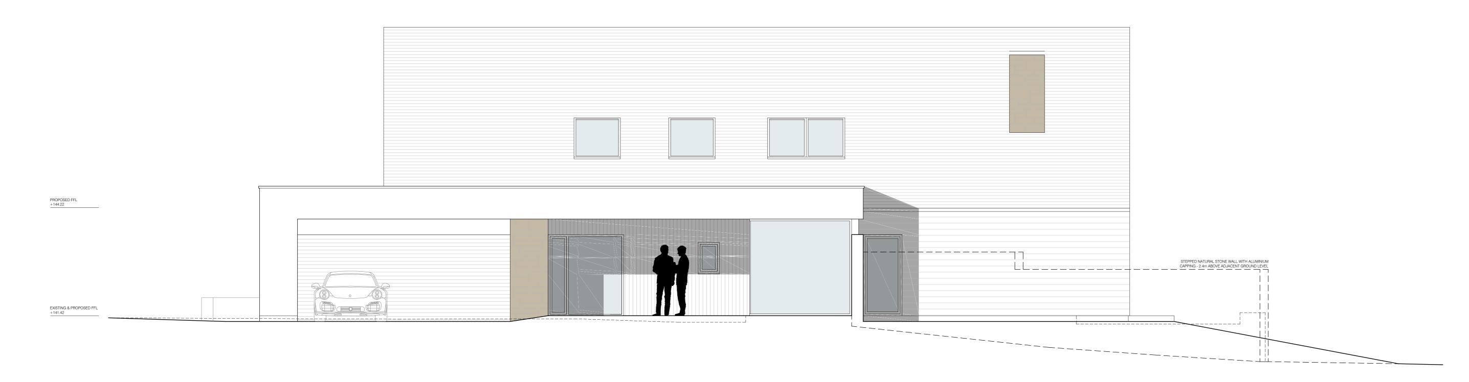
NATURAL SLATE CLADDING NATURAL TIMBER CLADDING NATURAL STONE WHITE SMOOTH RENDER VELUX ROOFLIGHTS FASCIA & SOFFIT GENERALLY: ALUMINIUM / PAINTED TIMBER & INTERNAL FACE OF DORMER ALUMINIUM / ALUMINIUM CLAD COMPOSITE FRAMED INSULATED POWDER COATED STEEL ROLLER DOOR POWDER COATED MATT BLACK REAR ELEVATION FLUE: FRONT GARDEN WALL:
