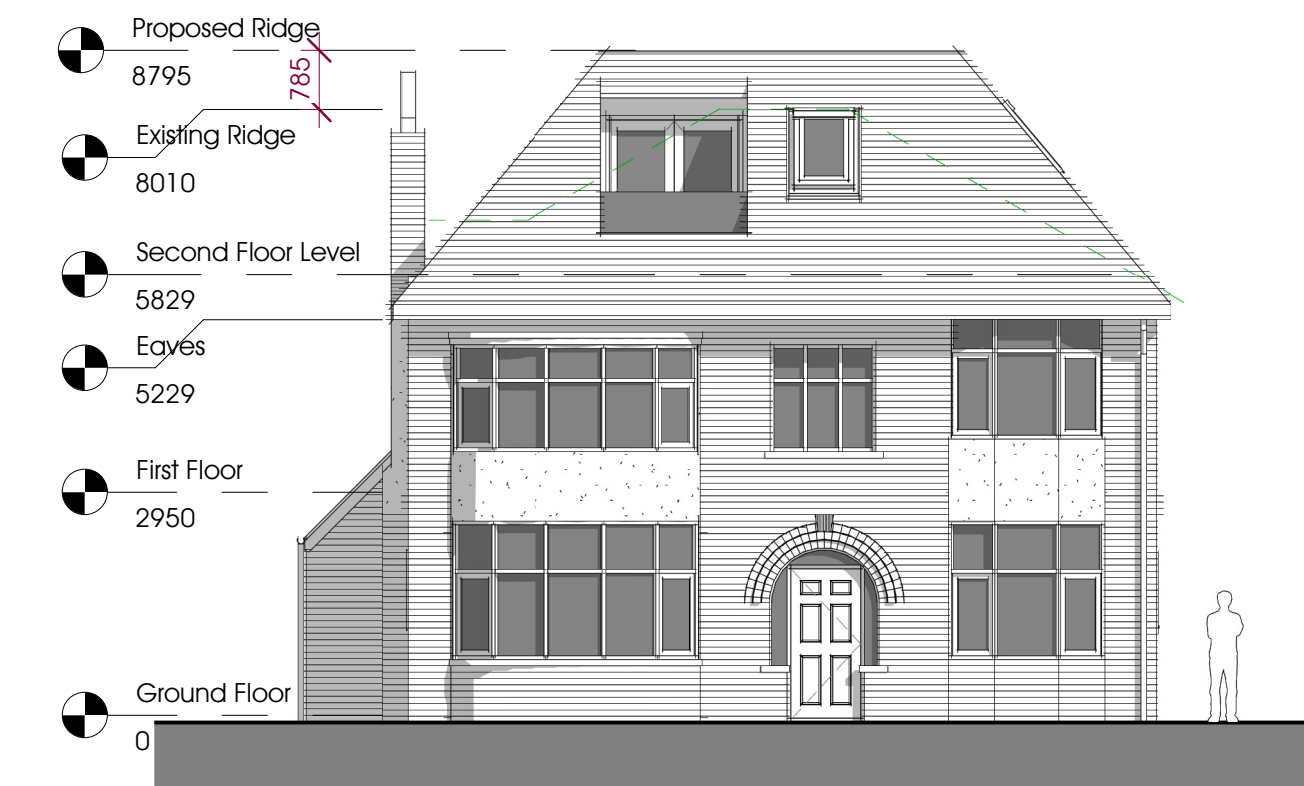
5 Proposed Front (north) Elevation 1 : 100
