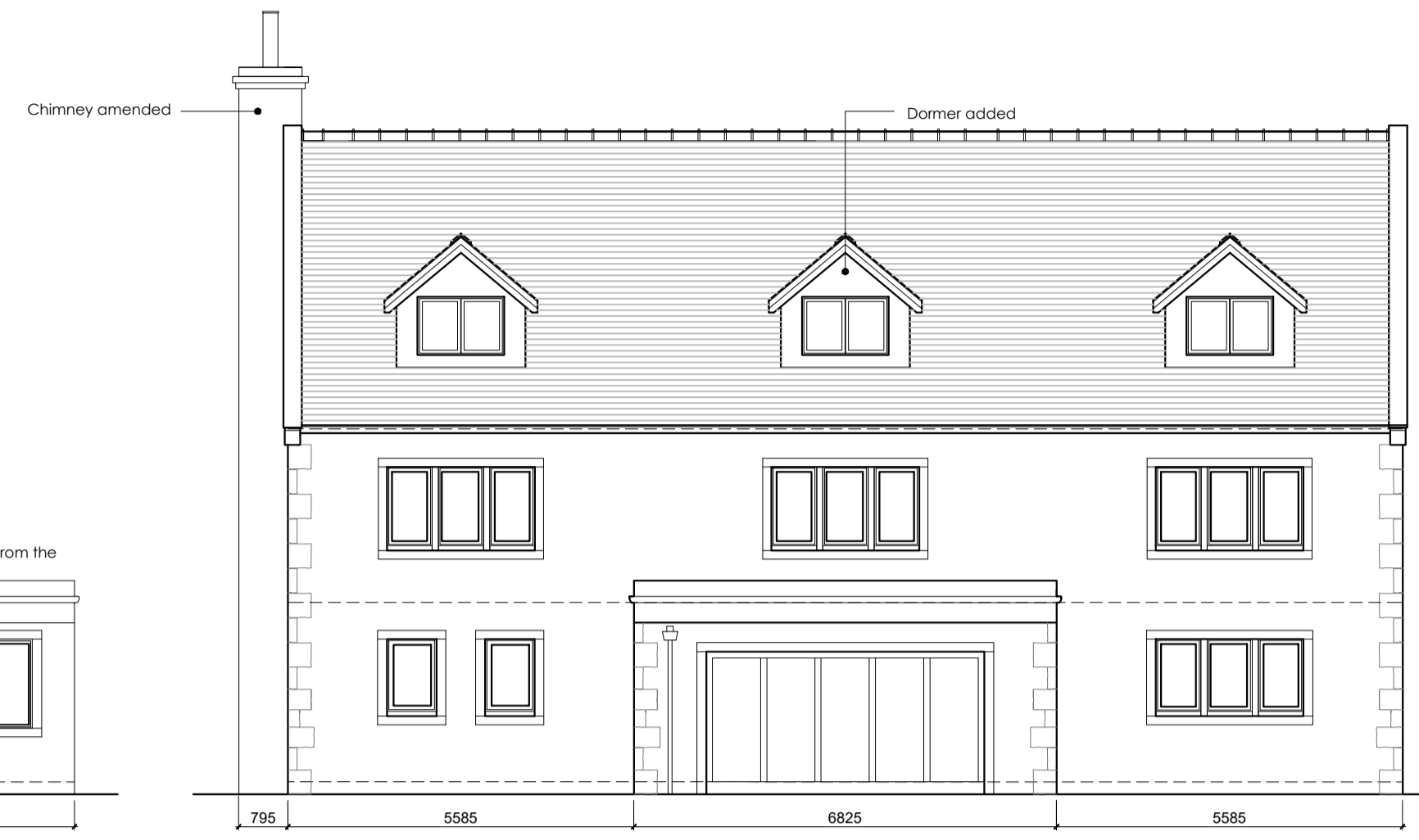
PROPOSED NORTH ELEVATION Scale 1:100
