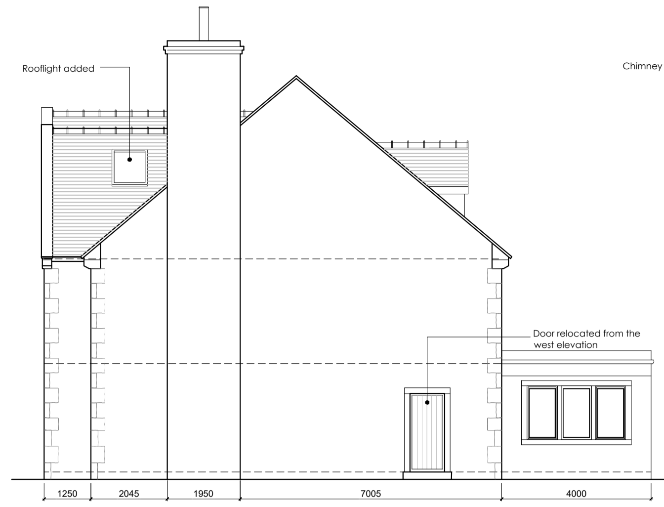
PROPOSED EAST ELEVATION Scale 1:100
