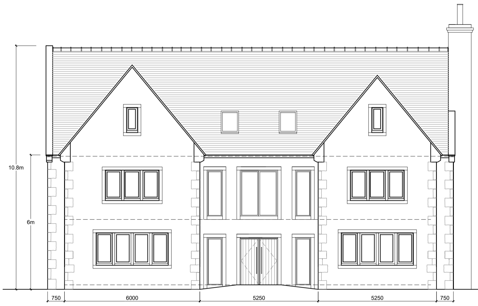
PROPOSED SOUTH ELEVATION Scale 1:100
