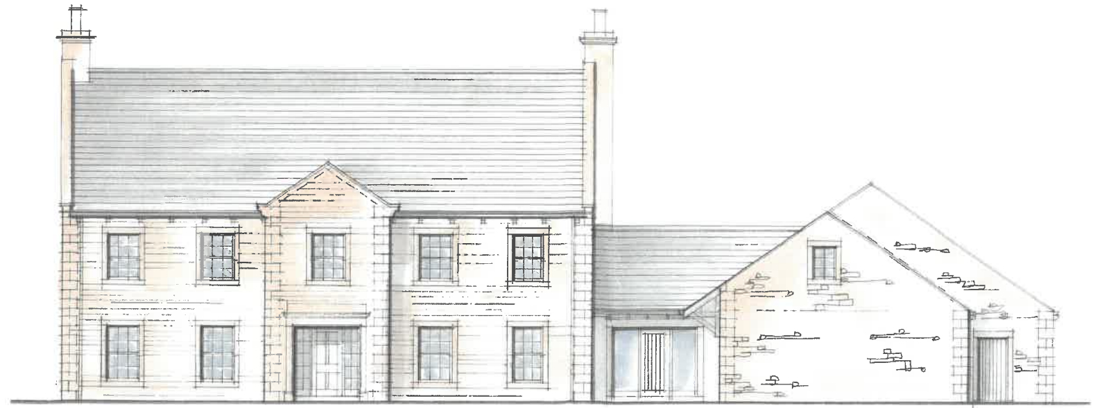
PL09: Extract from 6179-03A Current proposed north west elevation. Incorporating taller elegant sliding sash windows. NTS
