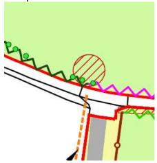
The plans show that long lengths of reinstated fencing are proposed. To minimise effects on the local landscape character this fencing should be of the timber post and wire stockproof type rather than post and rail which is proposed for the valve house compounds.
