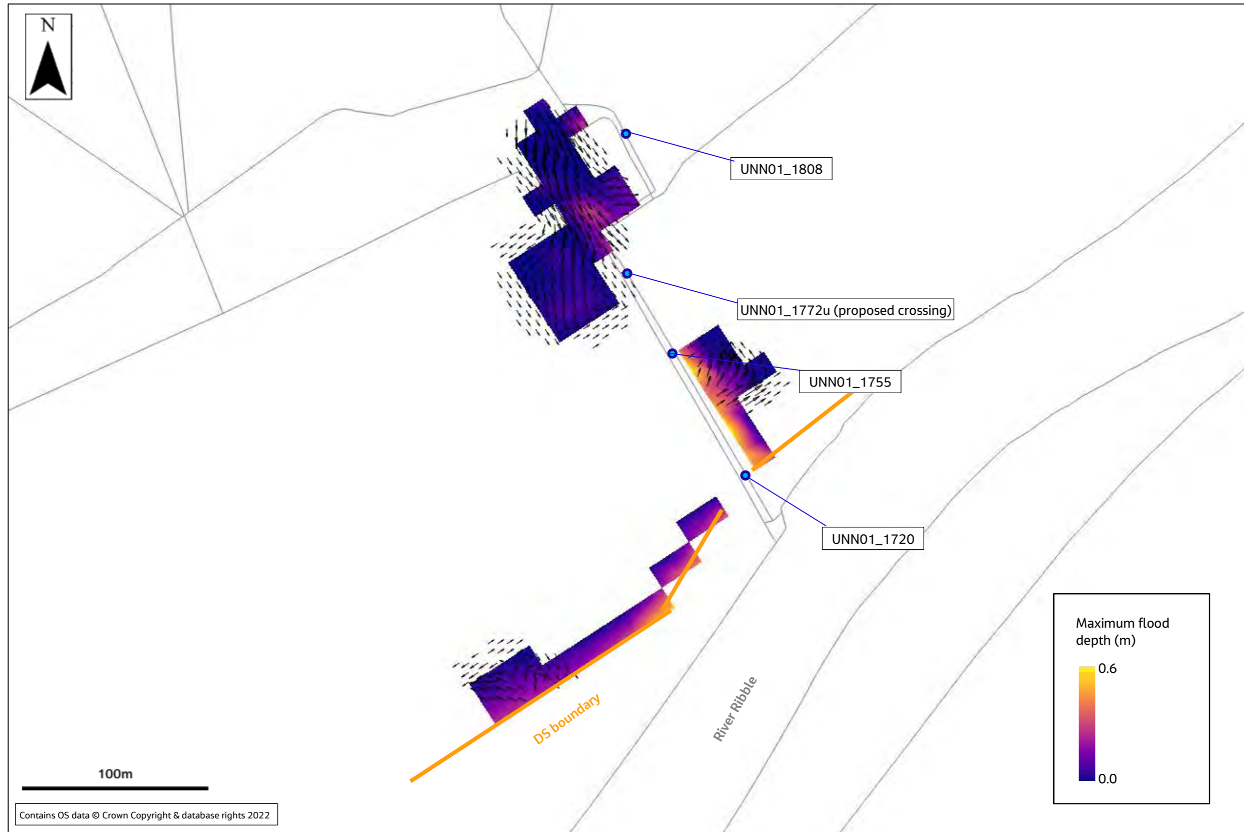
Figure 8-2: Unnamed Watercourse Baseline 1% AEP event modelled maximum flood depth and velocity vectors.
