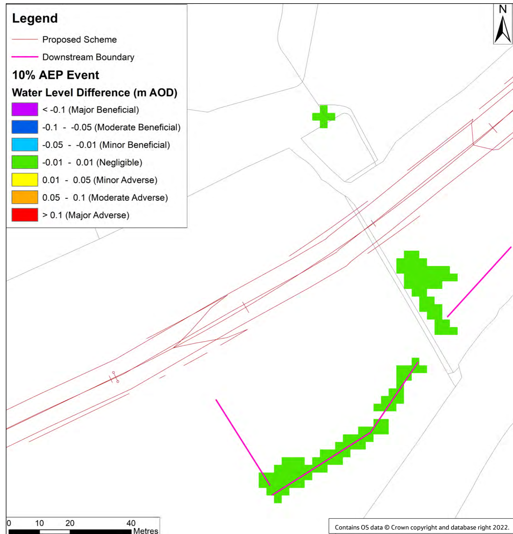
Figure E-9 Flood level difference map for the 10% AEP event. With-Proposed Ribble Crossing scenario minus baseline scenario.
