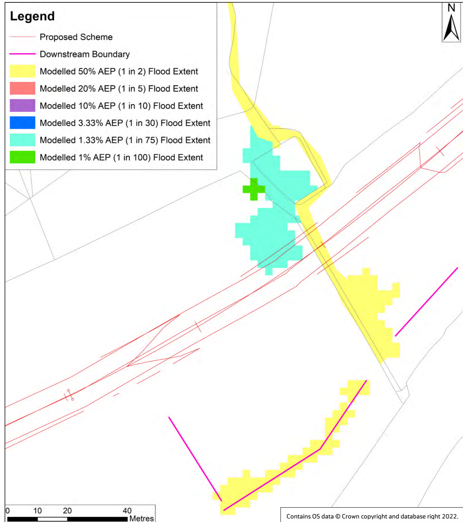
Figure D-2 Unnamed Watercourse Baseline modelled maximum flood extents, with proposed haul road footprint overlaid.
