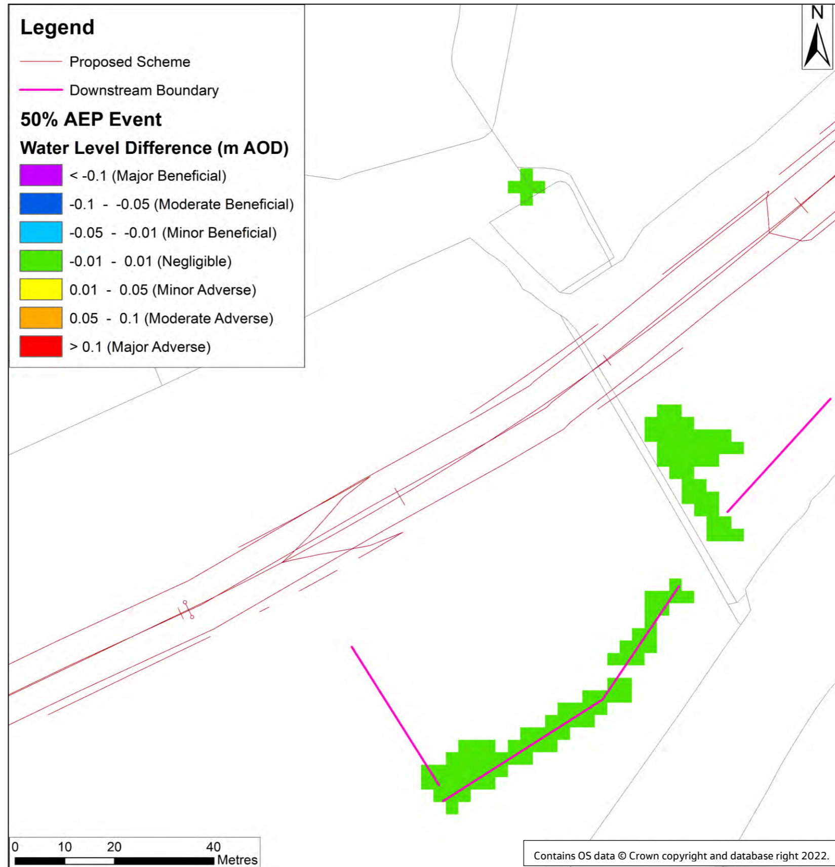
Figure E-7 Flood level difference map for the 50% AEP event. With-Proposed Ribble Crossing scenario minus baseline scenario.
