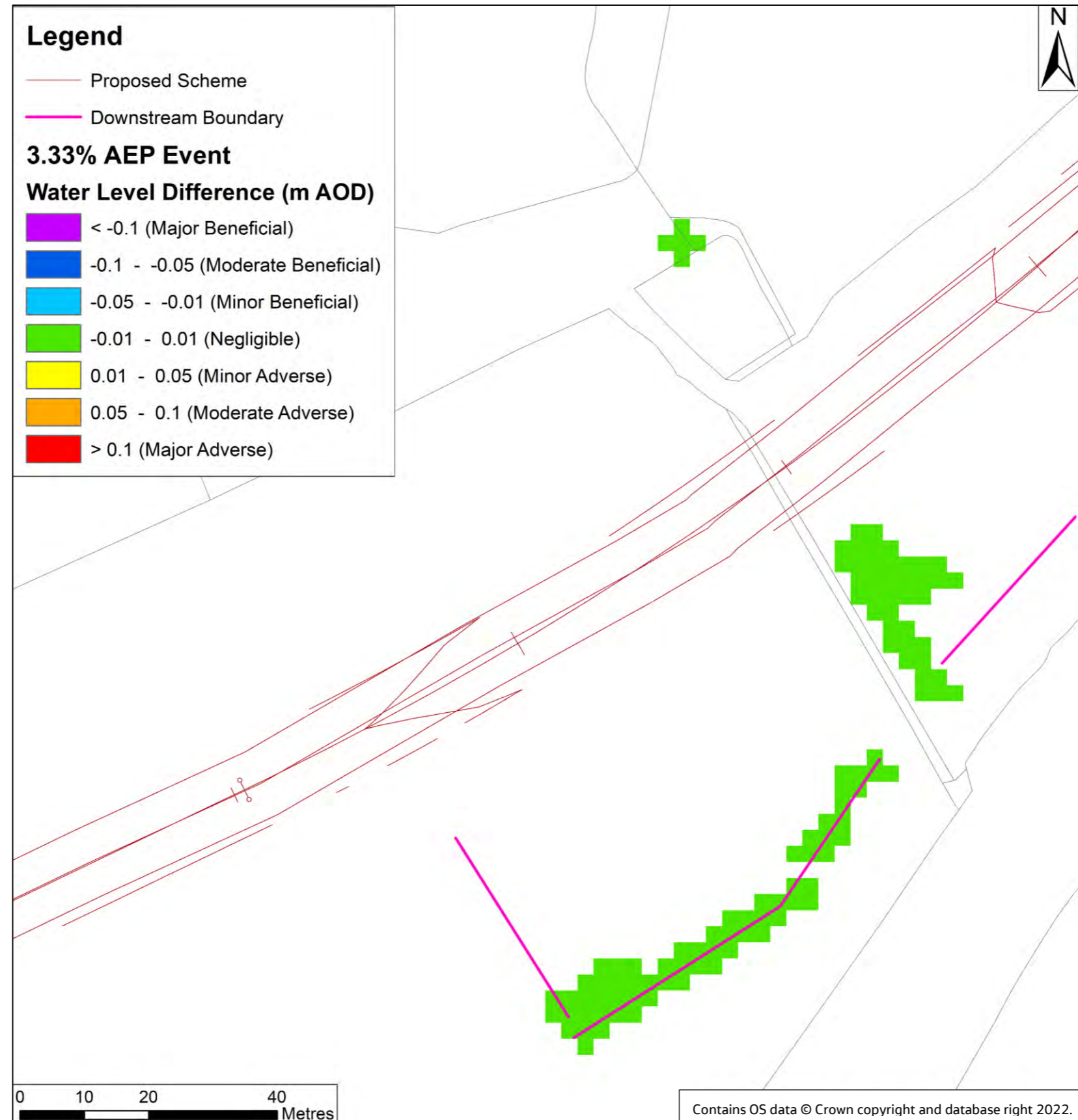
Figure E-10 Flood level difference map for the 3.33% AEP event. With-Proposed Ribble Crossing scenario minus baseline scenario.
