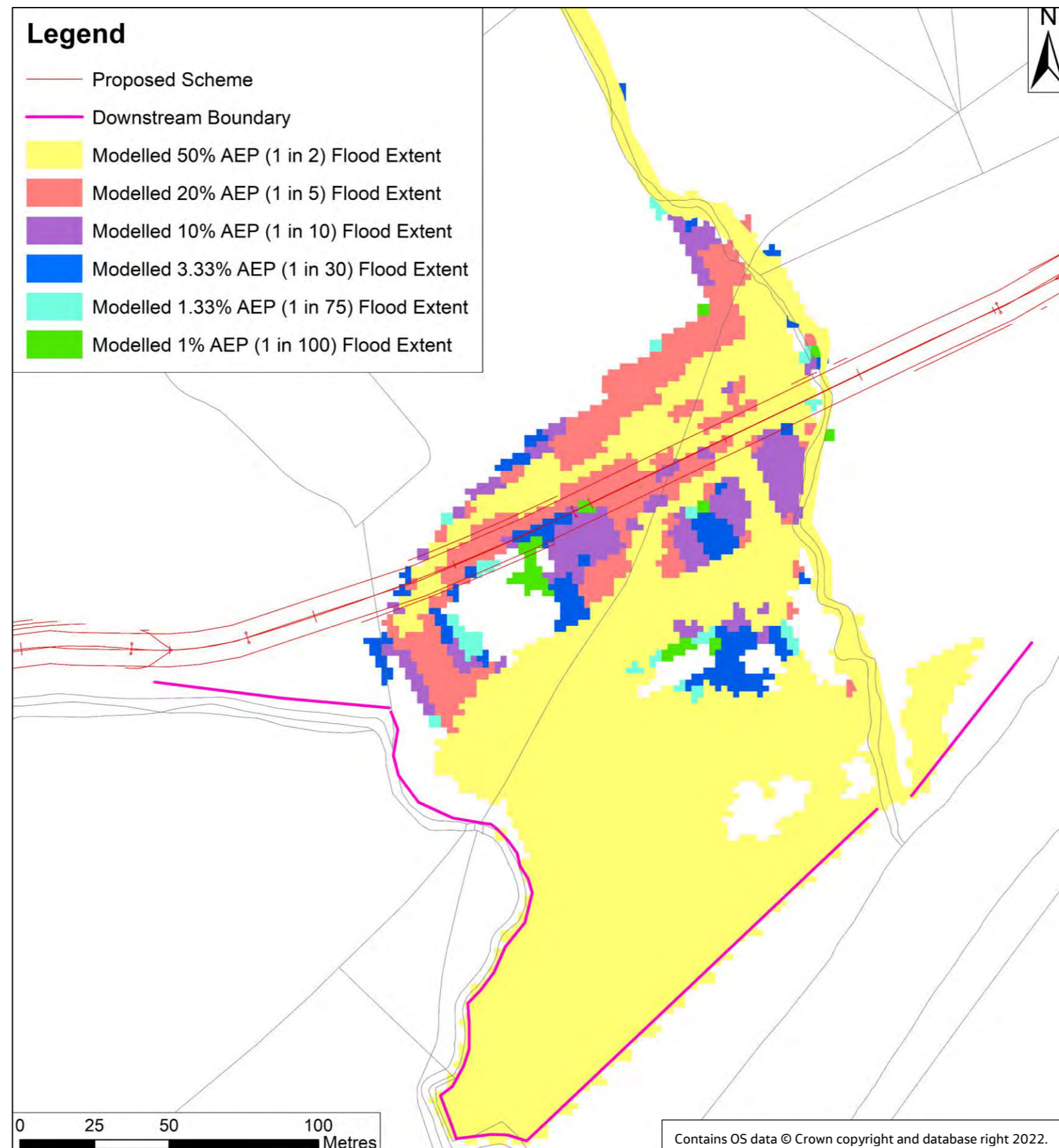
Figure D-3 Greg Syke Baseline modelled maximum flood extents, with proposed haul road footprint overlaid.
