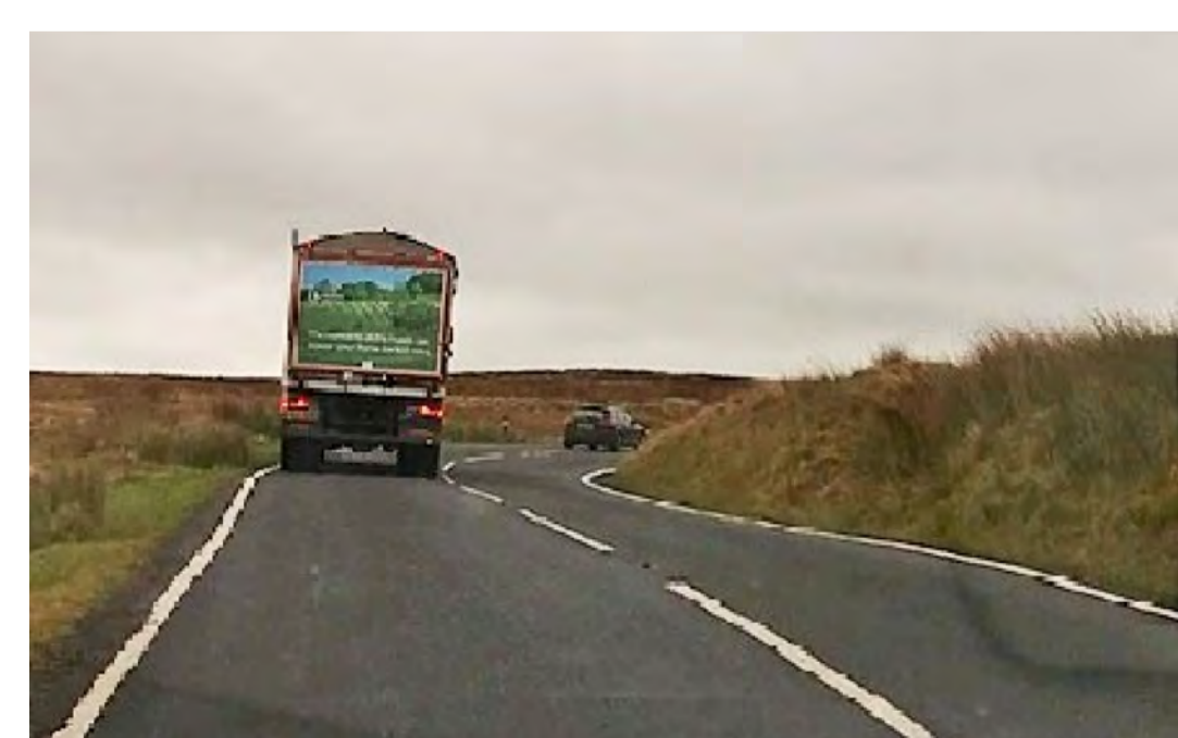
IMAGE 3: HGV TRIAL 11th NOVEMBER 2020 4AXLE RIGID TIPPER SLAIDBURN RD (SOUTHBOUND) TYPICAL OBSERVED LANE DISCIPLINE
