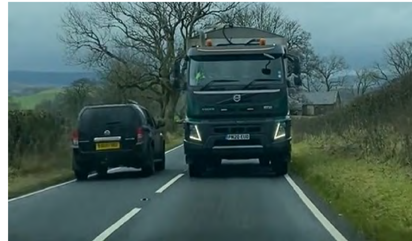
IMAGE 1: HGV TRIAL 11th NOVEMBER 2020 4 AXLE RIGID TIPPER HALLGATE HILL (SOUTHBOUND) TYPICAL OBSERVED LANE DISCIPLINE
