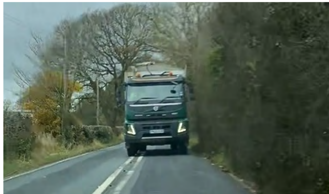
IMAGE 2: HGV TRIAL 11th NOVEMBER 2020 4 AXLE RIGID TIPPER SLAIDBURN ROAD (SOUTHBOUND) LEAVES LANE TO AVOID HEDGEROW
