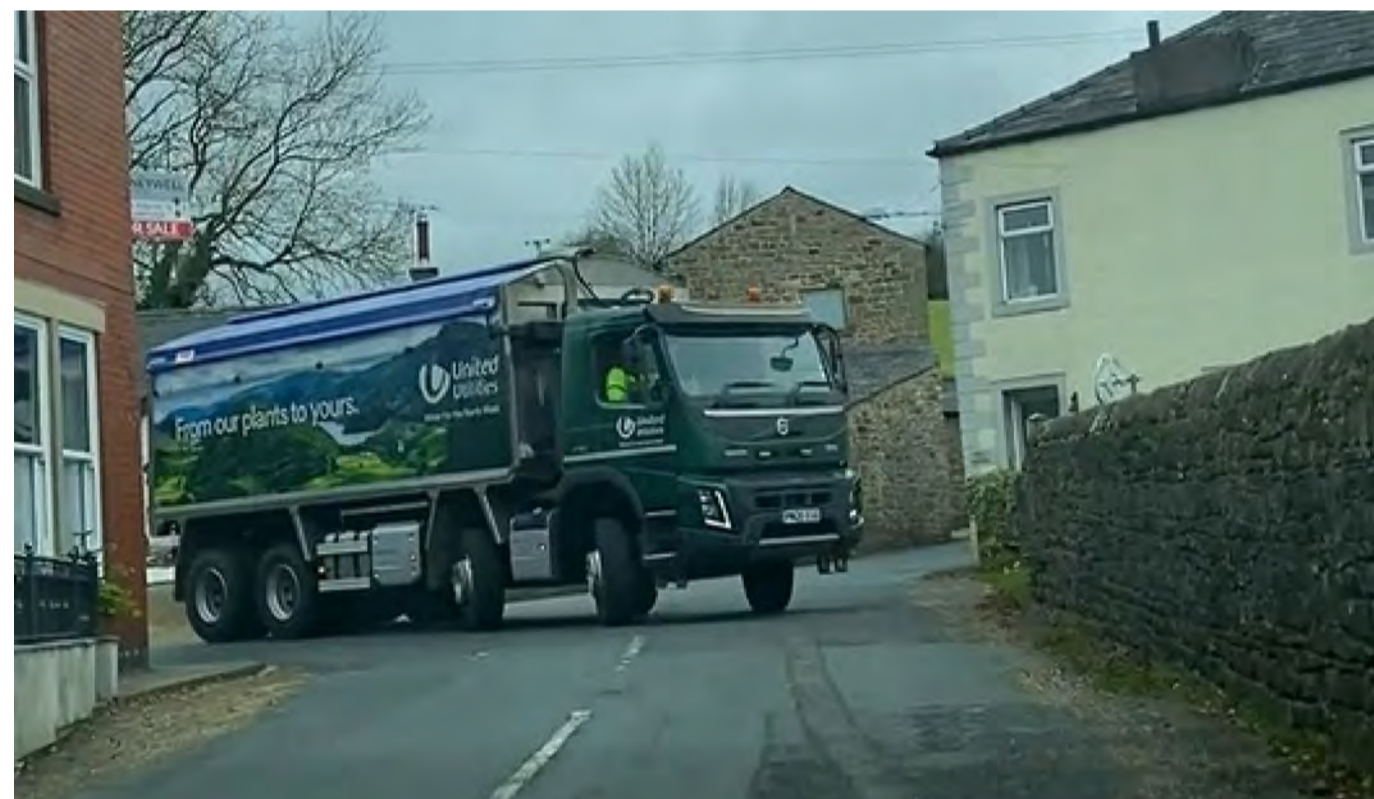
IMAGE 1: HGV TRIAL 11th NOVEMBER 2020 4 AXLE RIGID ENTERING EAST VIEW FROM GRINDLETON ROAD
