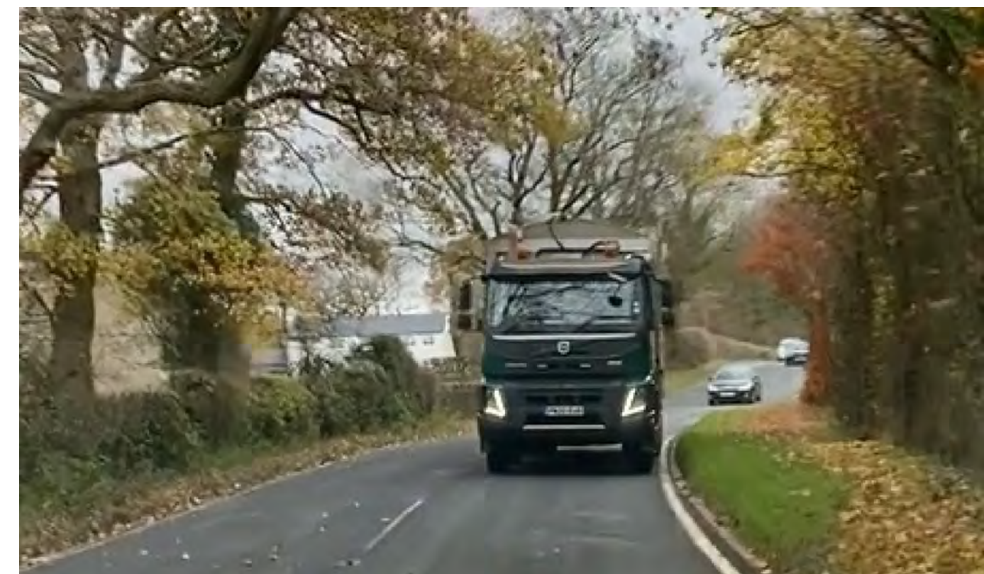
IMAGE 1: HGV TRIAL 11th NOVEMBER 2020 4 AXLE RIGID TIPPER SLAIDBURN RD (SOUTHBOUND) TYPICAL OBSERVED LANE DISCIPLINE
