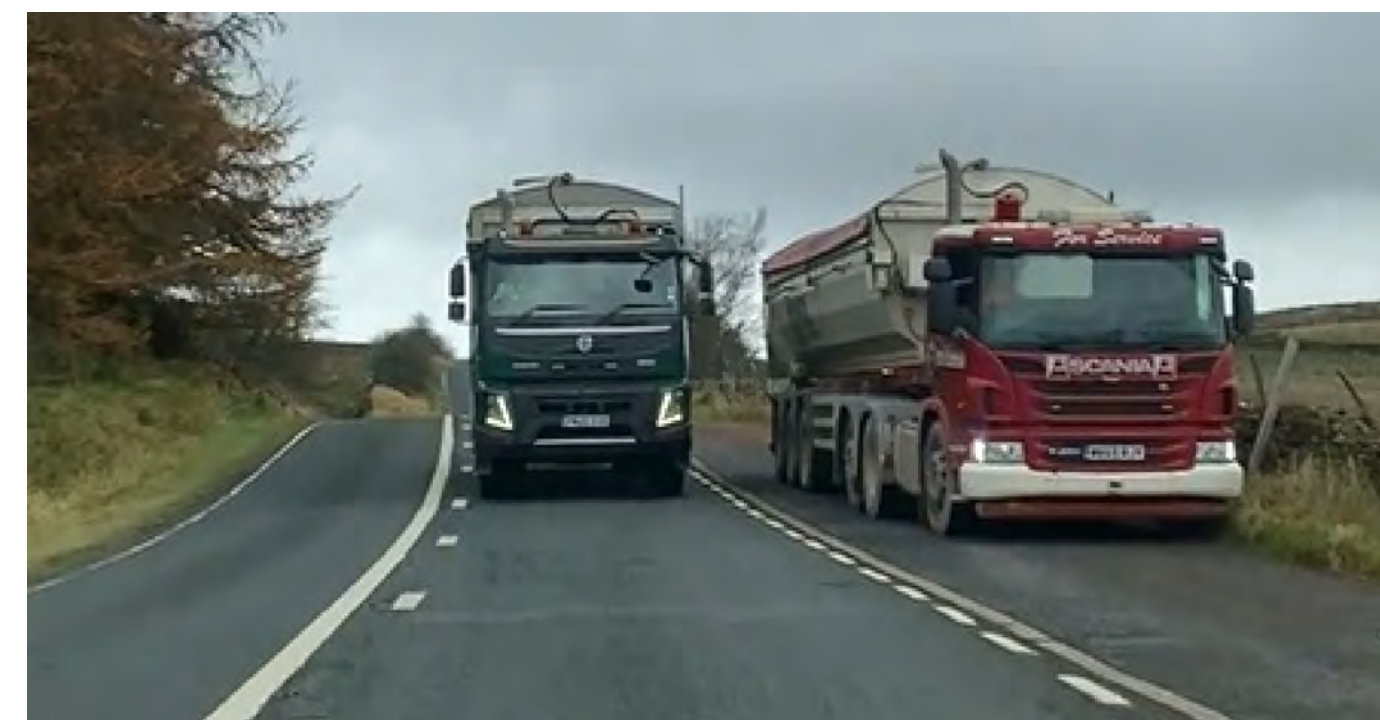
IMAGE 1: HGV TRIAL 11th NOVEMBER 2020 4 AXLE RIGID TIPPER SLAIDBURN RD (SOUTHBOUND) TYPICAL OBSERVED LANE DISCIPLINE
