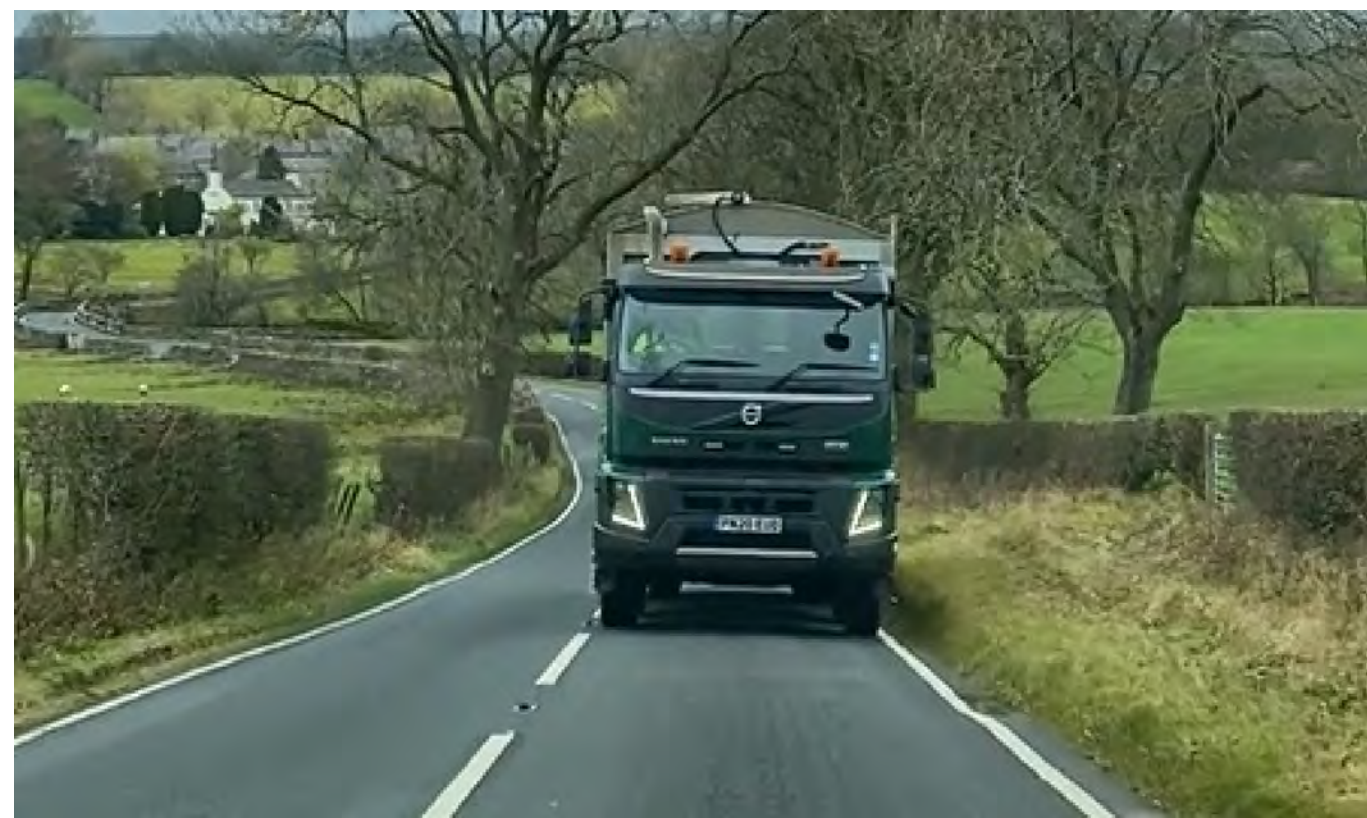
IMAGE 2: HGV TRIAL 11th NOVEMBER 2020 4 AXLE RIGID TIPPER HALLGATE HILL (SOUTHBOUND) TYPICAL OBSERVED LANE DISCIPLINE
