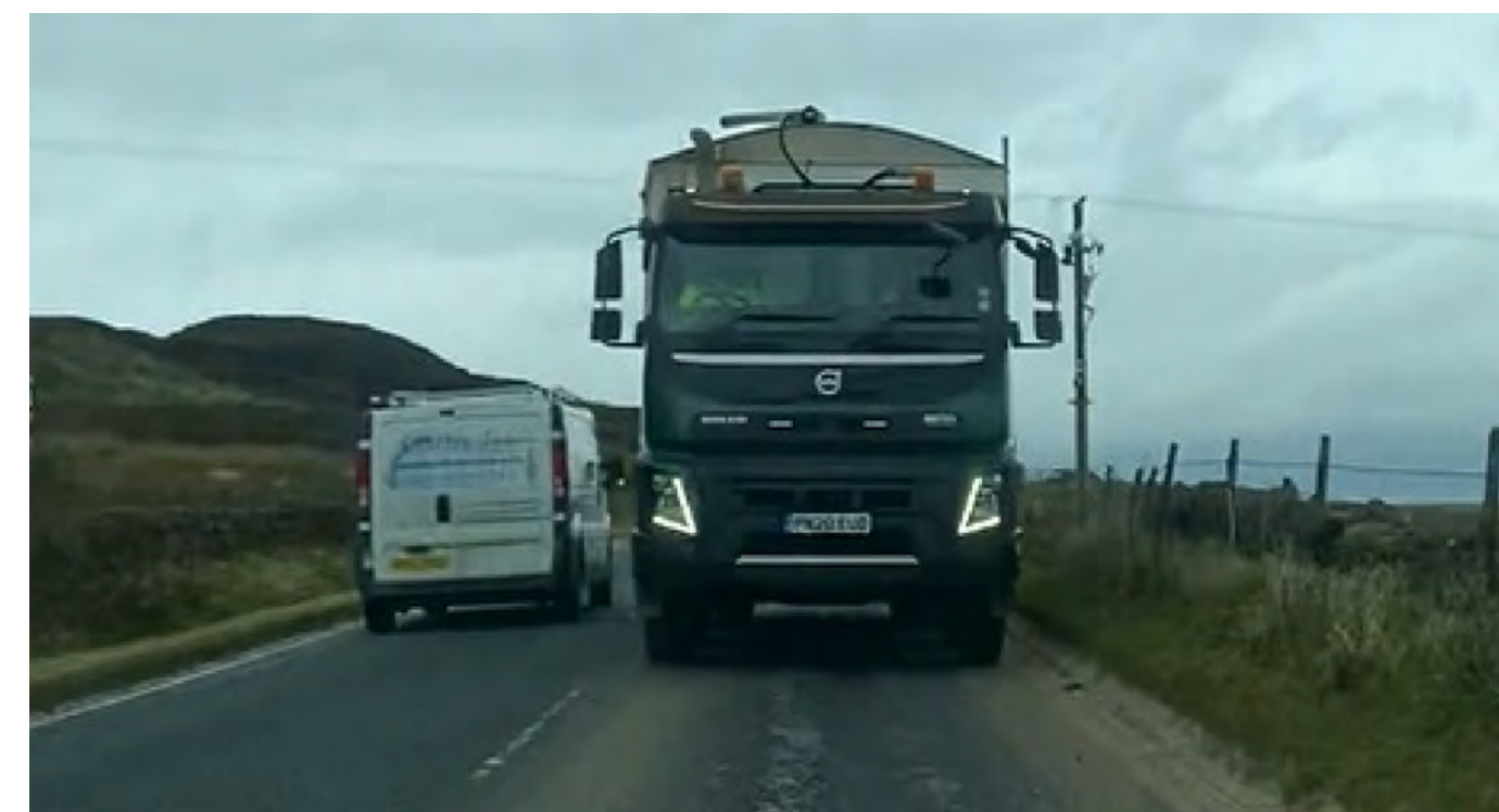
IMAGE 1: HGV TRIAL 11th NOVEMBER 2020 4 AXLE RIGID TIPPER HALLGATE HILL (SOUTHBOUND) TYPICAL OBSERVED LANE DISCIPLINE
