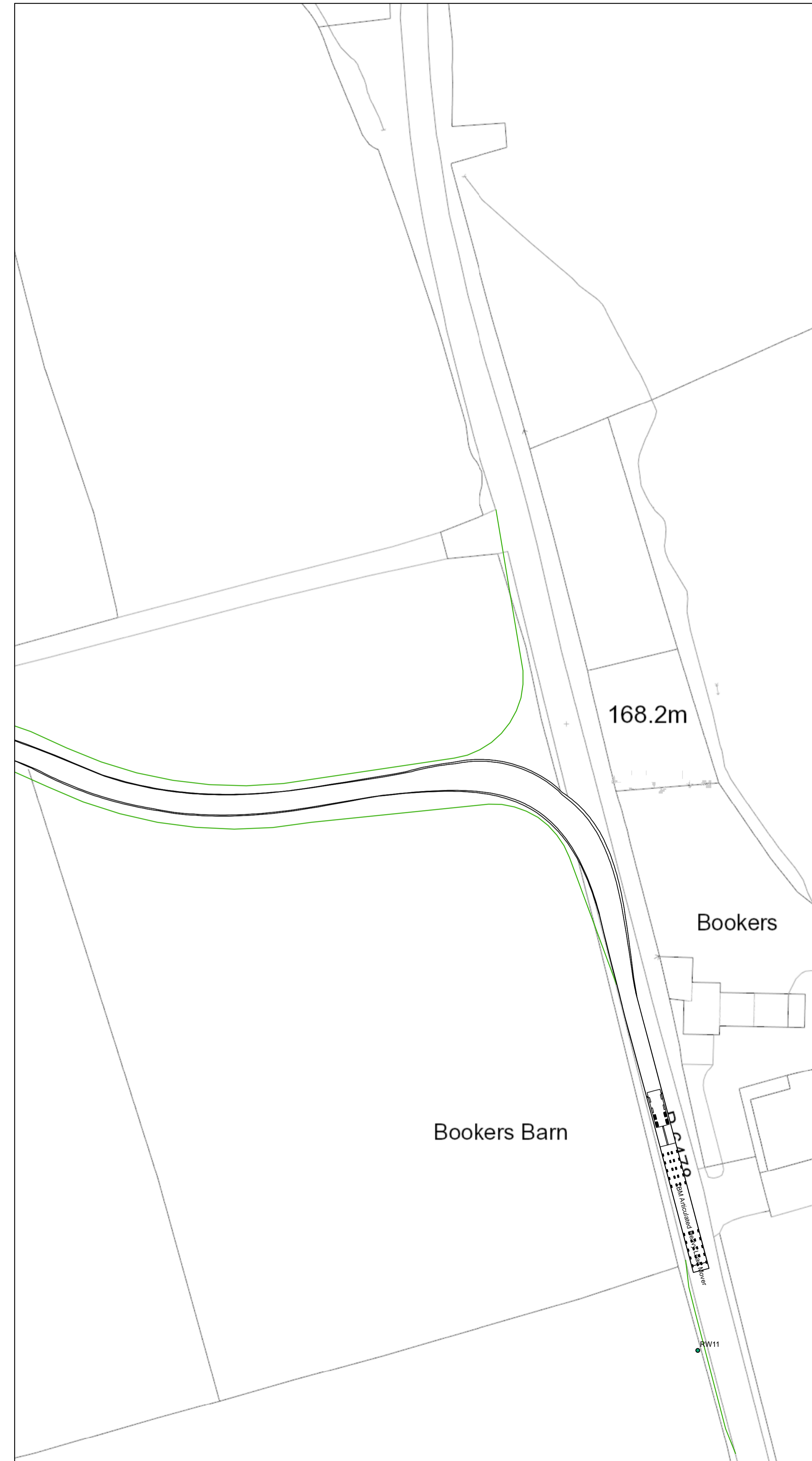
AIL - Tunnel Boring Machine Components to site (Southbound)
